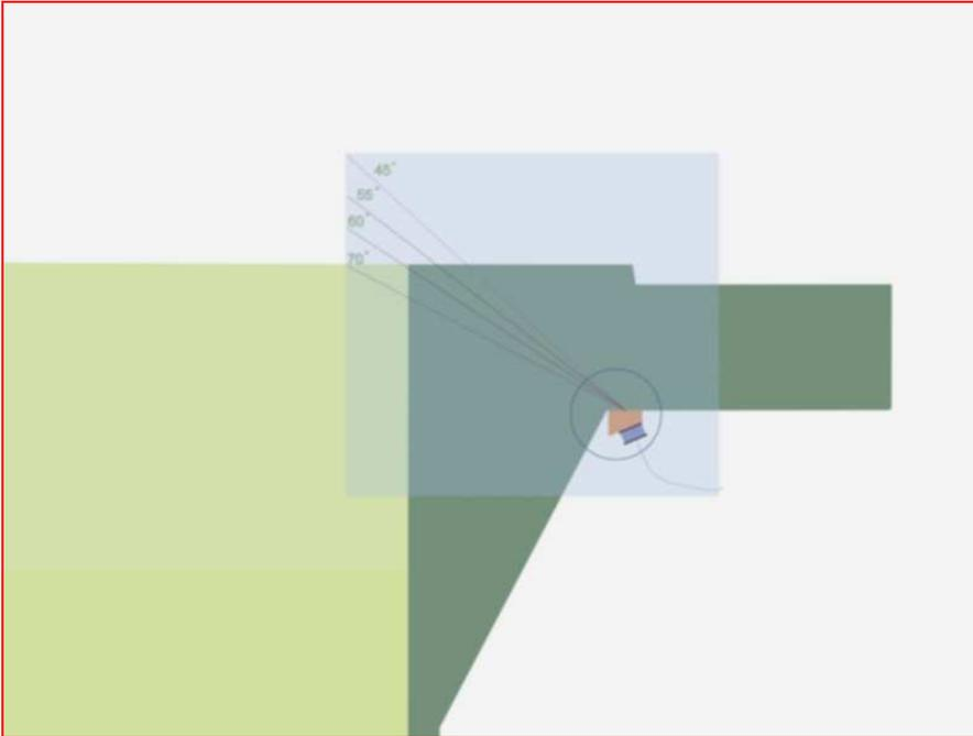
Figure -2: Beam Angle Selection using a Transparent Paper and 1:1 Scaled Flange Drawing
