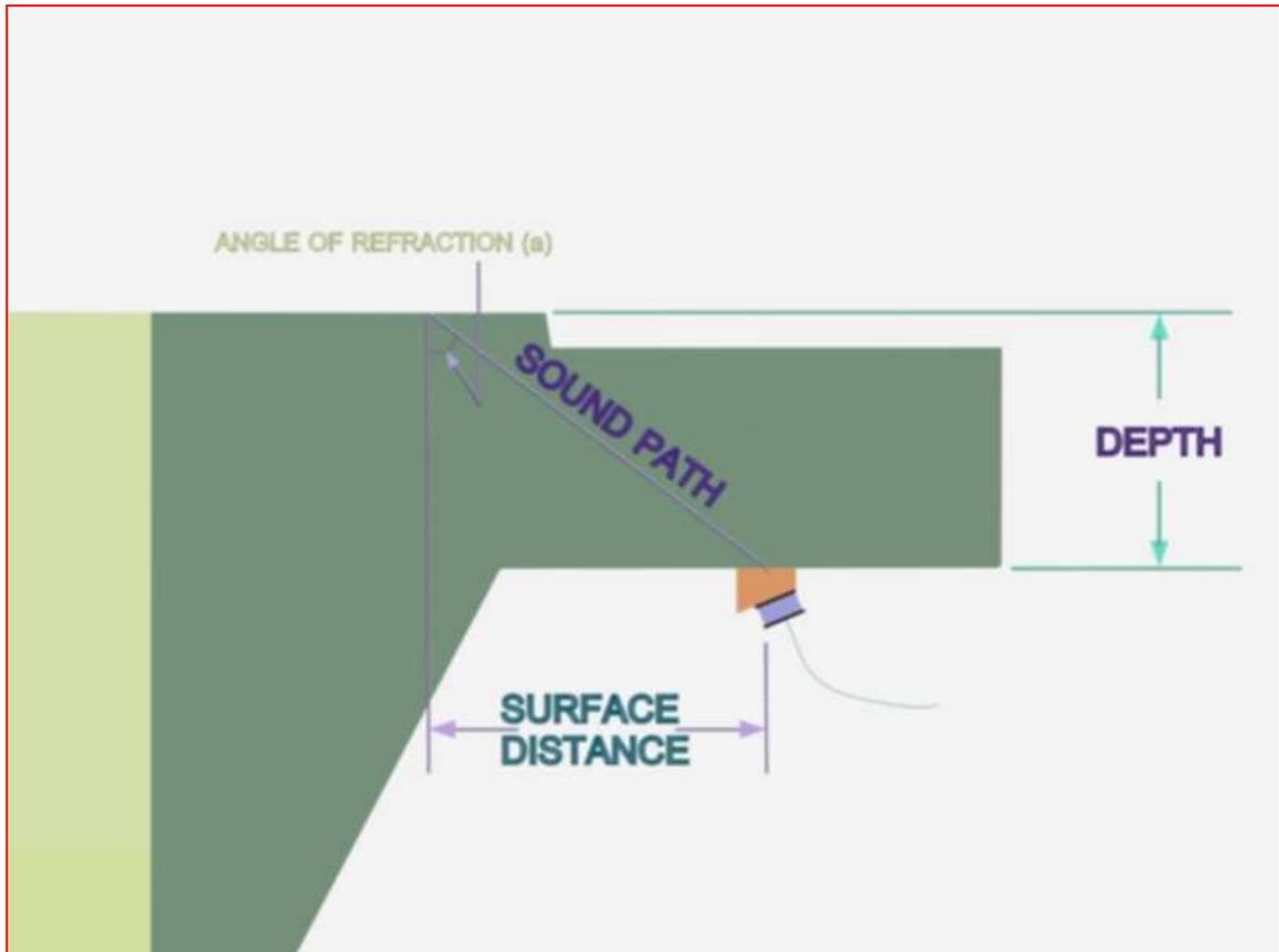
Figure – 3: A 2D Drawing Showing Required Dimensions to be Identified
