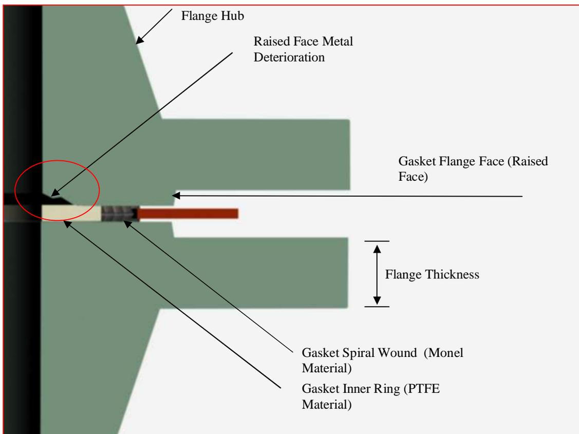
Figure – 1: A Close View for 2 WN Flanges Connected with Spiral Wound Gasket Showing a Metal Attack from Process Side (note: bolts are not shown)
