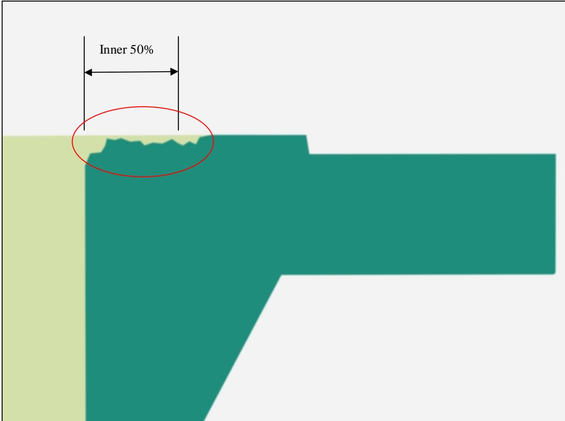
Figure – 4: Rejected Flange due to Corrosion more that 50% of the Flange Face
