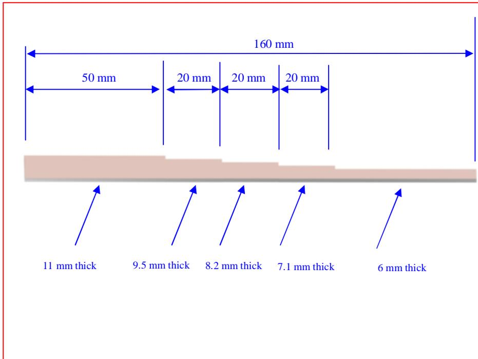
Figure - 5: Side View of the Curved Step-Wedge with Dimensions
