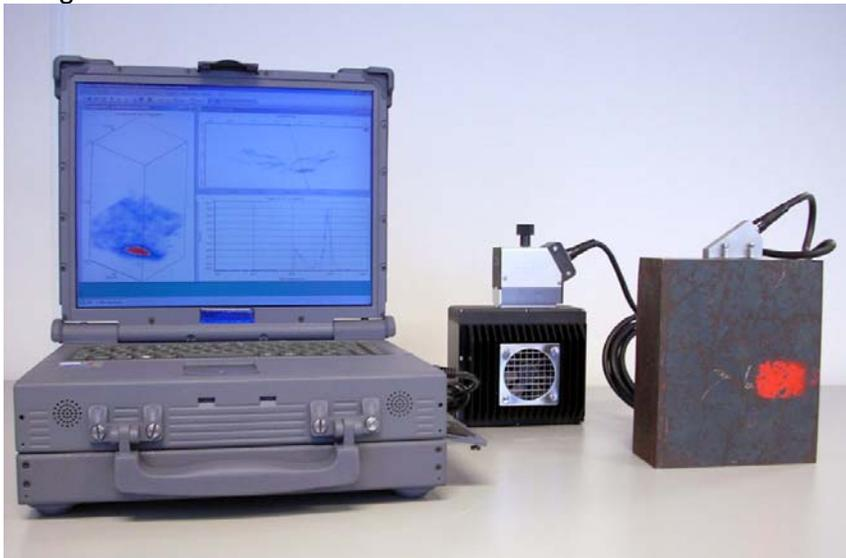
**Figure 7: Sonovision Sampling Phased Array system**
