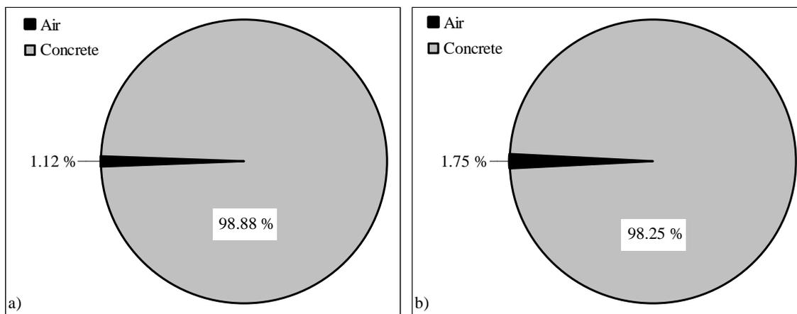
**Figure 8 Percentage of volumes of concrete and air, a) base and b) top.**
