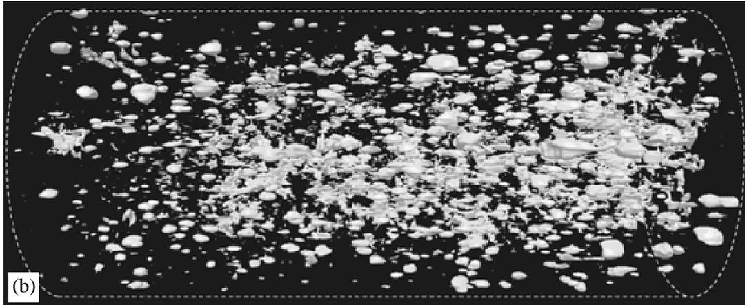
**Figure 5 Structure of air pores within the scanned sample, a) top, b) base**
