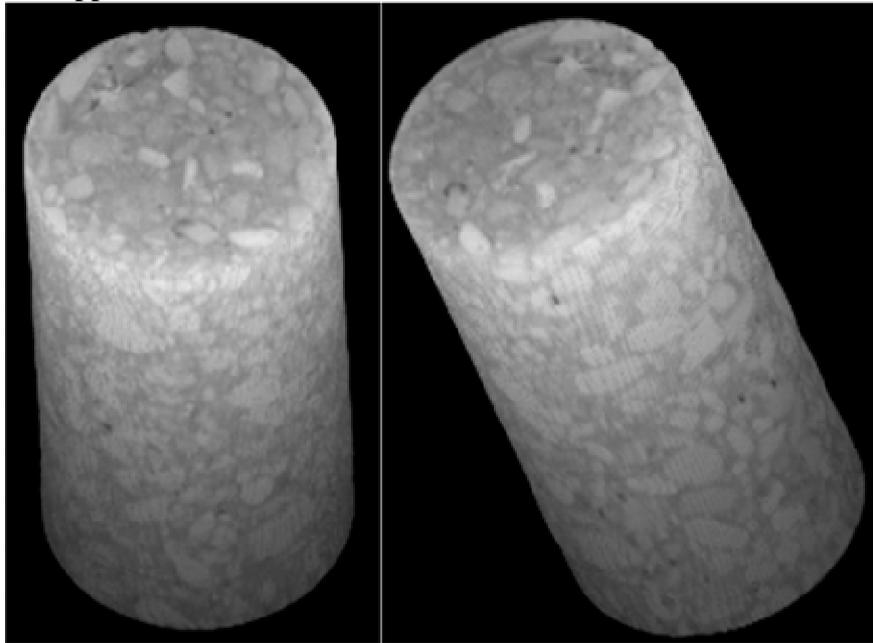
**Figure 4 Reconstructed 3-D view of concrete core specimen (base)**
