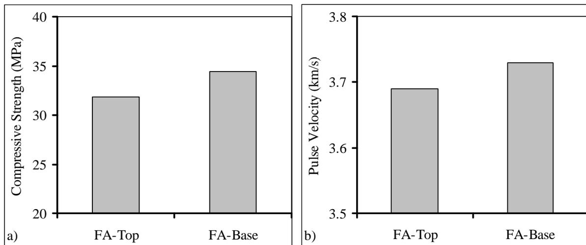
**Figure 6 a) Compressive strengths and b) UPV values of specimens from different locations**
