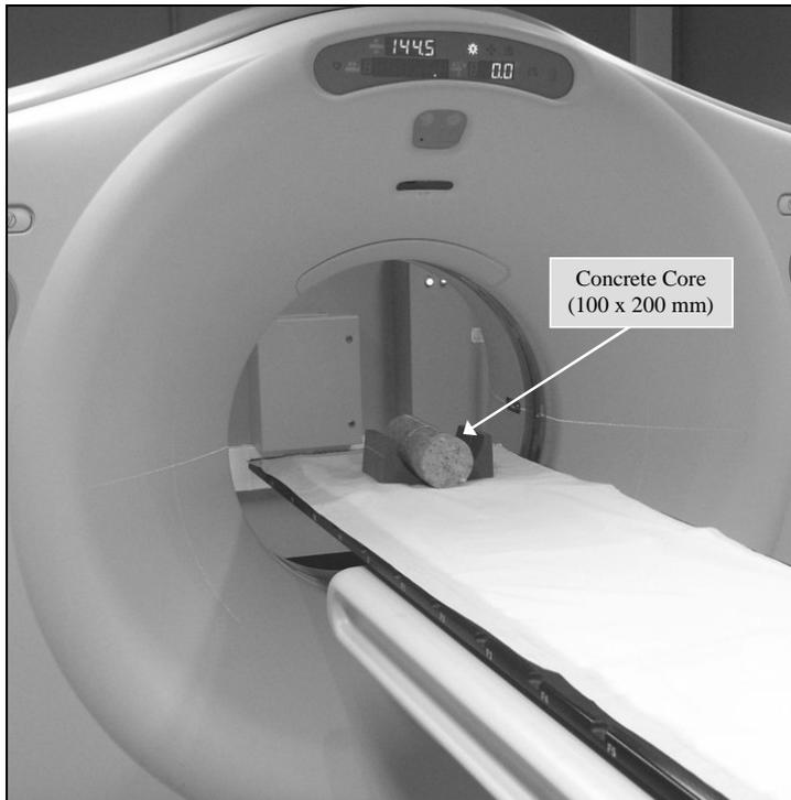
**Figure 2** A general view of the CT machine during concrete core scanning.
