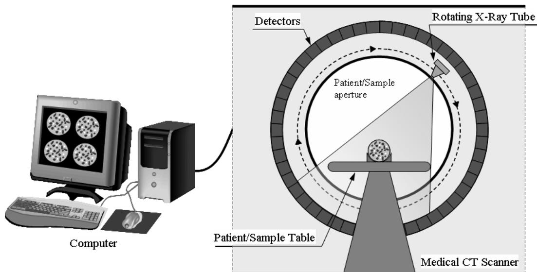
**Figure 3** Schematic explanation of how a CT scanning system works.
