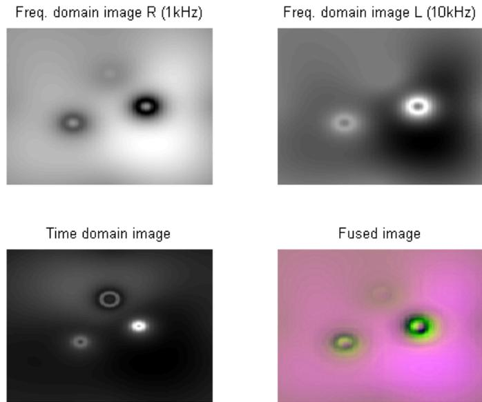
Fig. 5. Fusion obtained with wavelet decomposition, where the high spatial resolution image  $T$  is frequency domain image.
