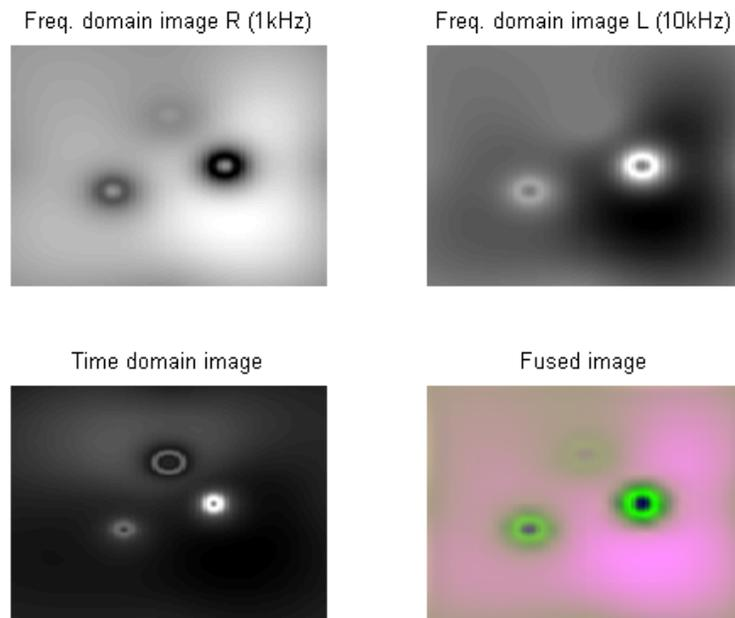
Fig. 6. Fusion obtained with wavelet decomposition as described, where the high spatial resolution image  $T$  is time domain image.
