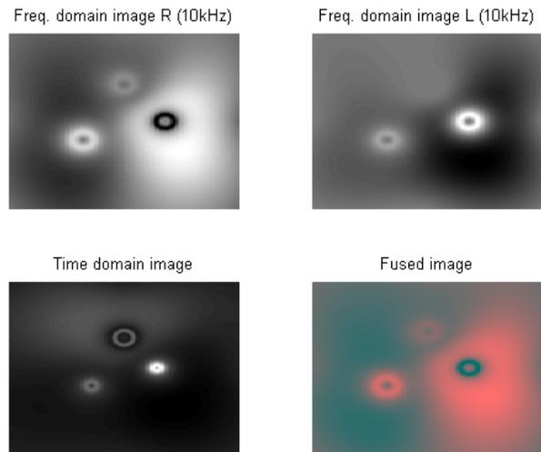
Fig. 3. Simple fusion, with 2 frequency domain images and one time domain image.
