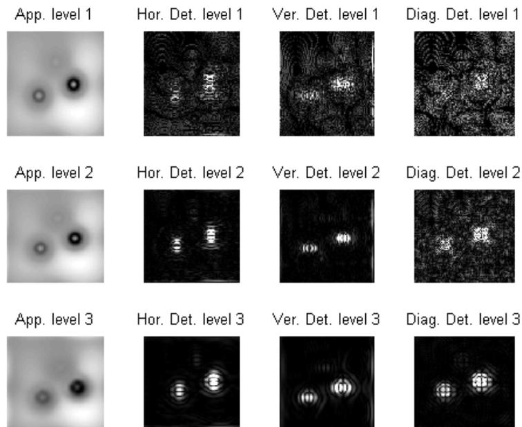
Fig. 8. Approximation and detail coefficients of image  $T''$ . Daubechies wavelets are used.
