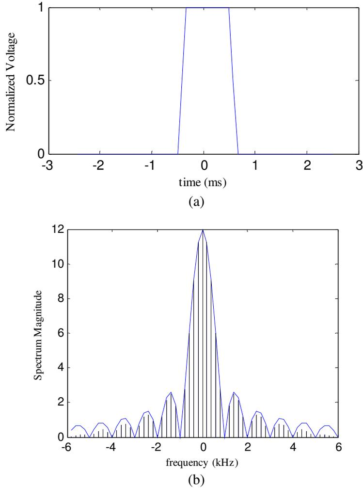
Fig. 1. Typical PEC excitation pulse in time domain (a) and spectrum of frequency domain (b).
