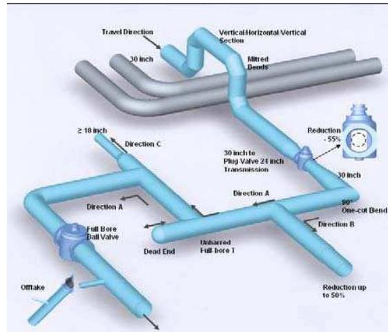
**Figure 1. Typical piping configuration as design basis for the ROBOT**
