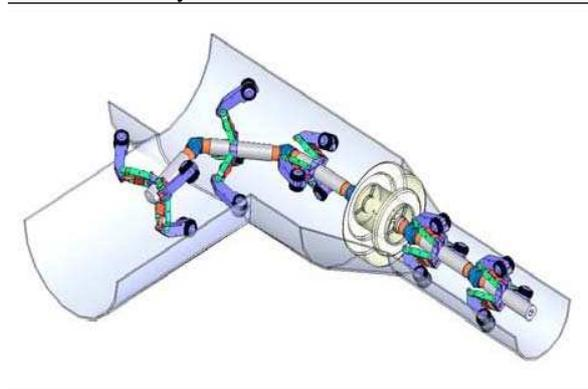
**Figure 6. RoBot entering Off-Take. Shown is also the use of the Power-Generation-Module (expanded to maximize turbine driving flow)**
