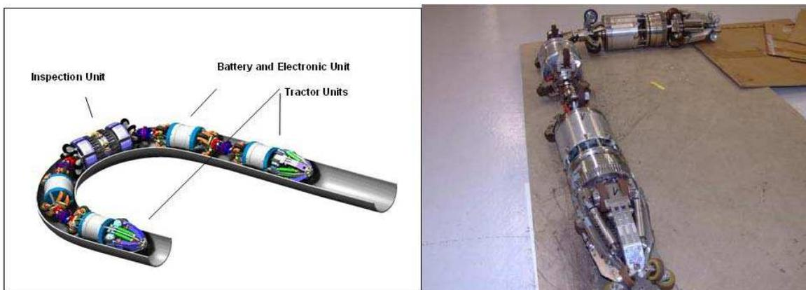
**Figure 7. Robotic Test System (RTS). Optimized for autonomous inspection of vertical venting pipelines.**
