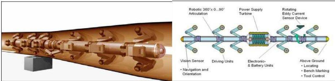
**Figure 5: Final concept of the Robotic Inspection Tool**
