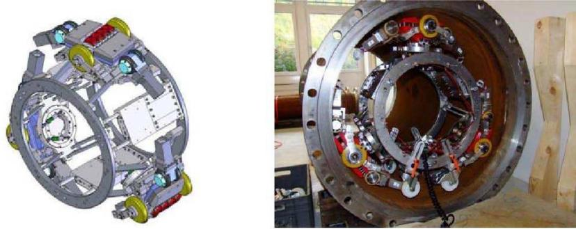
**Figure 10. Self driven corrosion detection tool**
