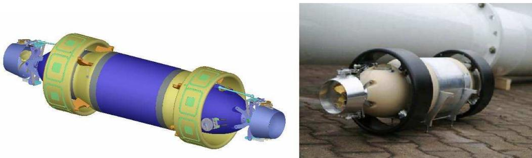
**Figure 9. RoFloat: Free swimming leak detection tool**
