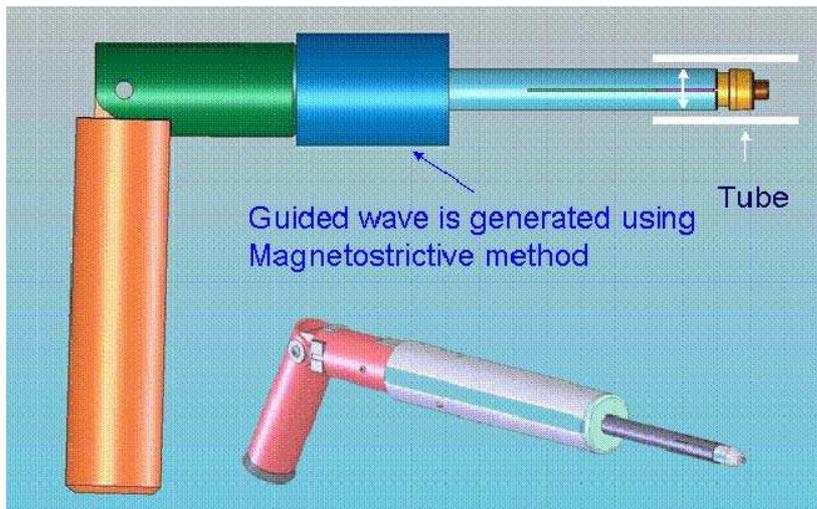
For long-range guided wave inspection and monitoring, a short pulse of guided waves in relatively low frequencies (up to a few hundred kHz) is launched along the structure under inspection, and signals reflected from geometric irregularities in the structure such as welds and defects are detected in the pulse-echo mode. From the time of flight of the defect signal and the signal amplitude, the axial location and approximate severity of the defect are determined.
