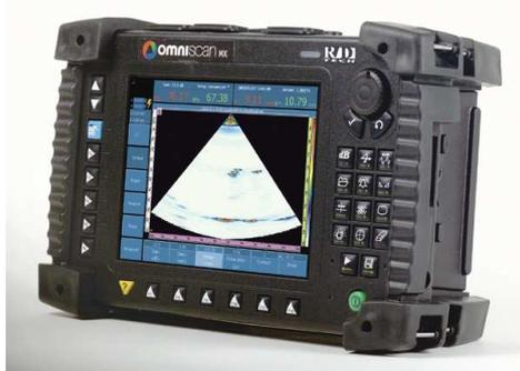
**Figure 1 Photo of Olympus NDT OmniScan performing an L-wave S-scan.**
