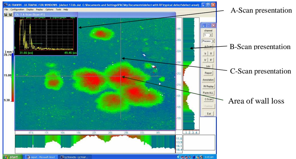
Figure 4: Example of a typical area of wall loss (red in color).
