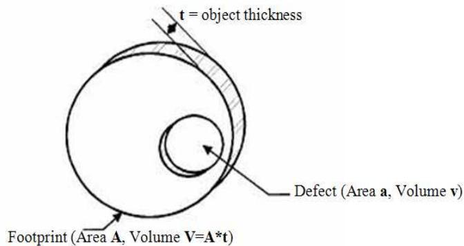
Fig. 7 Defect detection within footprint
