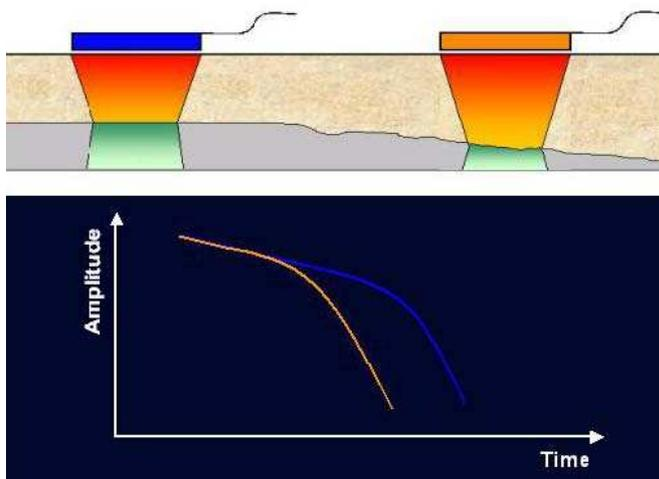
Fig. 5 RTD-INCOTEST signal, shorter signal on corroded area
