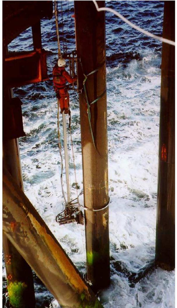
Fig. 3 RTD-INCOTEST on riser with upsailer
