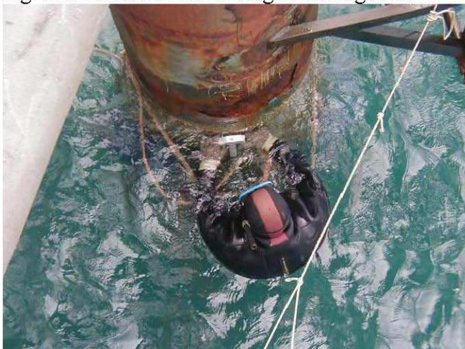
Fig. 2 RTD-INCOTEST on riser with diver
