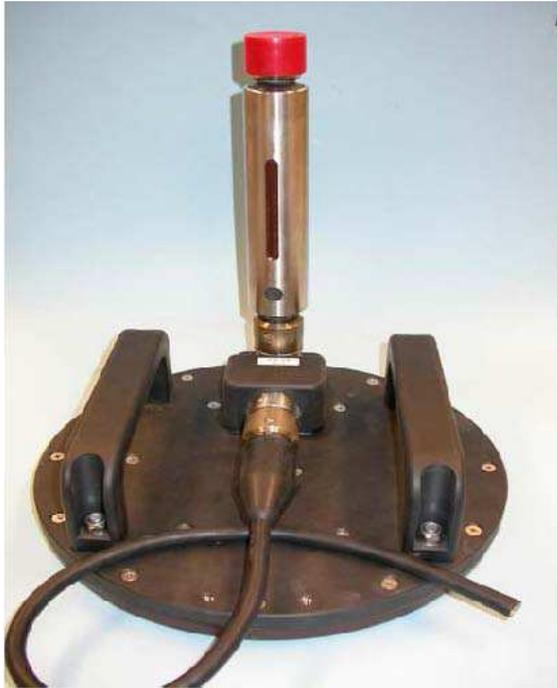
Fig. 11 RTD-INCOTEST Subsea probe designed for operation at -2000m (Test pressure 250Bar)
