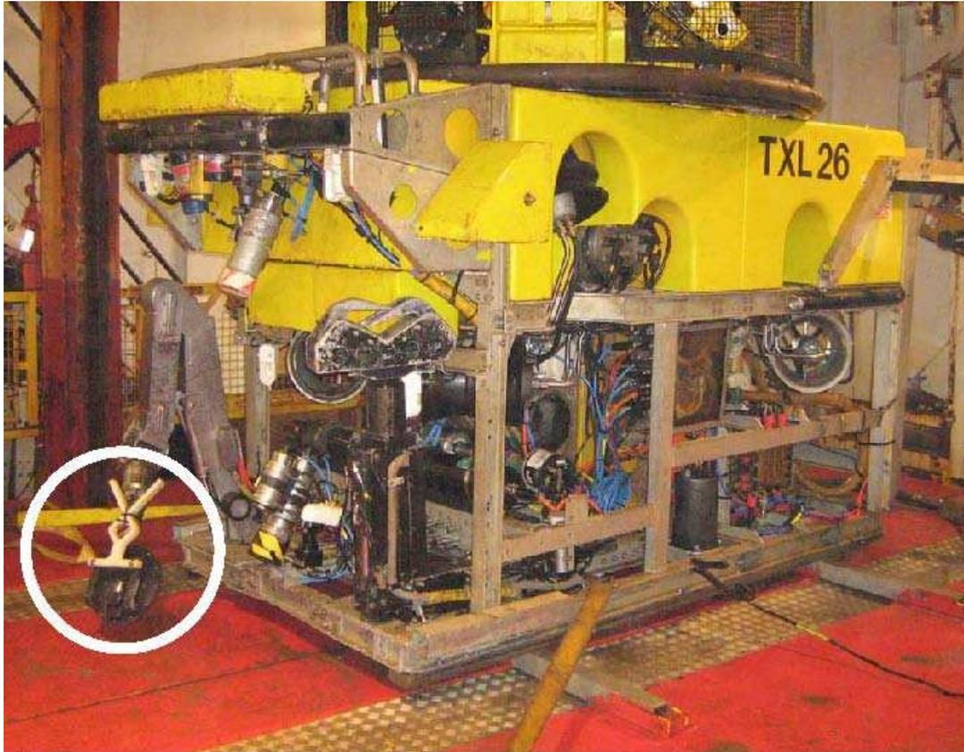
Fig. 12 RTD-INCOTEST Subsea probe on WORK CLASS RO
