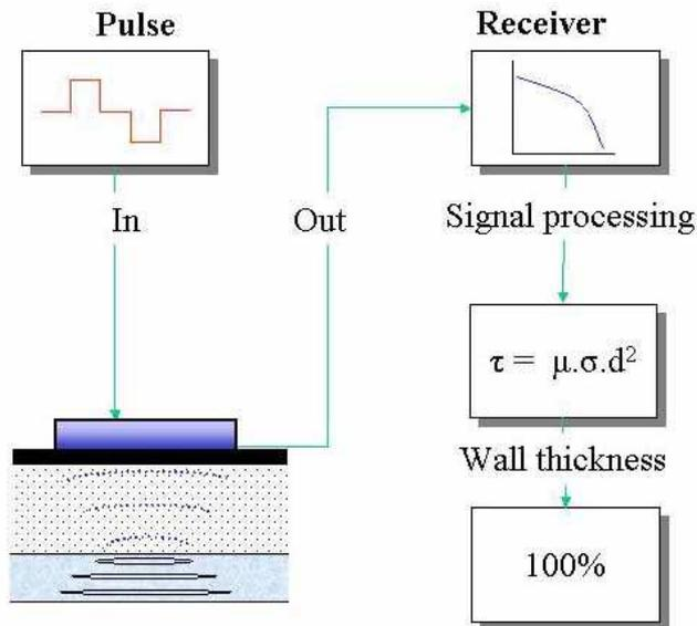
Fig. 6 RTD-INCOTEST Pulse-Receiver schematic
