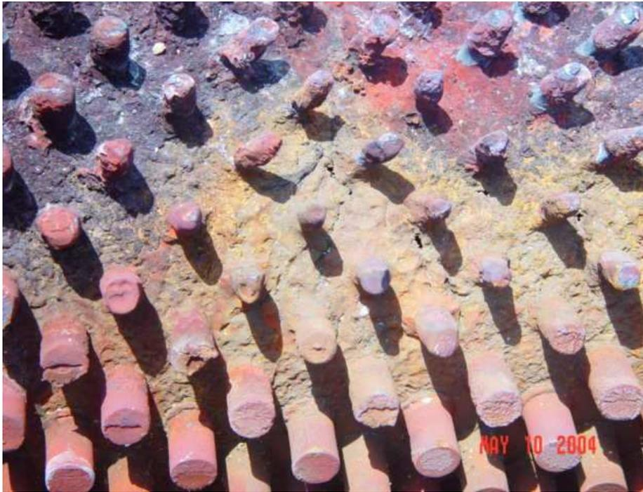
**Figure 5. Convection Pipe With External Corrosion**
