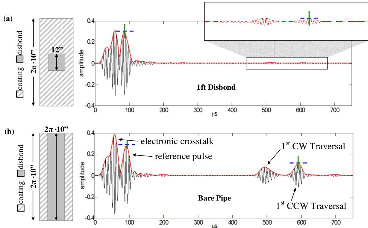
Figure 2: Ultrasonic waveforms obtained from a 20"-diameter schedule 10 pipe with a coal-tar wrap coating with a (a) 1ft. disbond and for a (c) bare pipe. The SH1 modes was used at a frequency of 130kHz.
