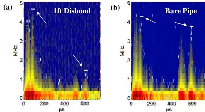
Figure 3: STFTs of RF-waveforms for a (a) 1ft disbond and a (b) bare pipe. A 64-point Hanning window with 32-point overlap was used.
