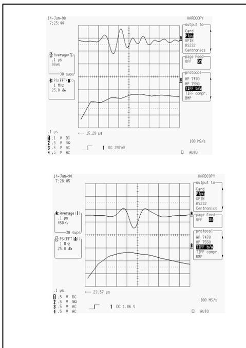
Specific equipment in the form of an oscilloscope and pulser/receiver, with the added requirement that the oscilloscope be equipped with signal averaging and Fast Fourier Analysis is normally required although this can be performed on any computer with the required software as long as the "A" scan can be averaged, digitized and saved. A 10 Mhz, 0.375" broadband compression wave transducer is used for spot measurement. No
