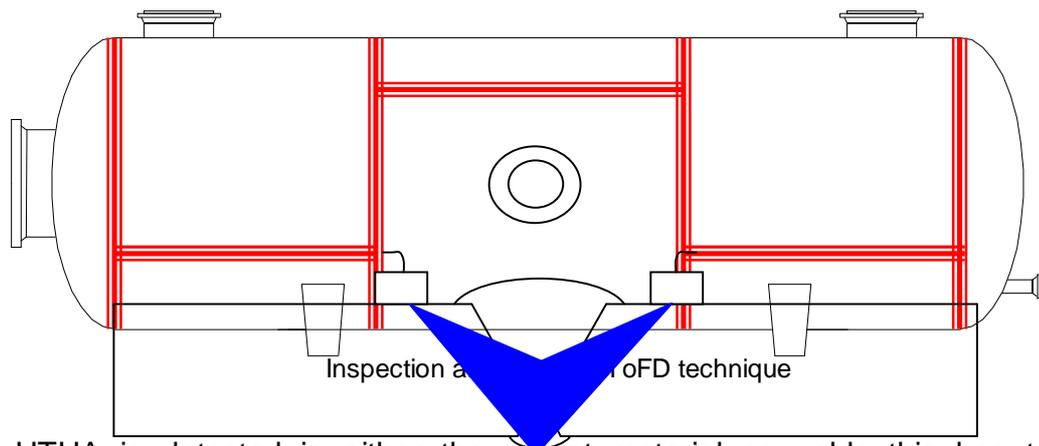
Where HTHA is detected in either the parent material or welds this has to be confirmed by secondary ToFD – All longitudinal and circumferential weld seams when HTHA and inclusions or other impurities. This is a two step approach and consists of Velocity Ratios and Fast Fourier Transformation techniques. Where no evidence of HTHA is detected by the primary inspection technique the inspection is considered complete.
