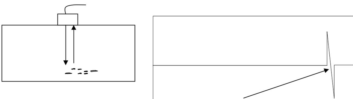
The primary detection technique is the pattern based back scattering technique and involves the use of a normal UT flaw detector with a 0 degree, 1/2", 5Mhz broadband, longitudinal wave transducer. Suspect areas are scanned and the ultrasonic signal shape is observed for evidence of "scatter" from the grains as depicted in Figure 1.
