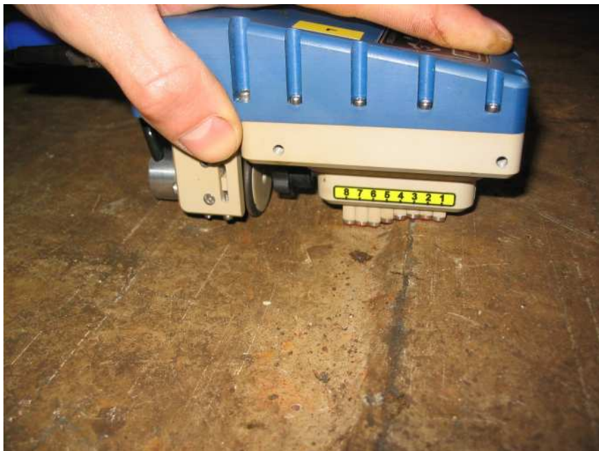
Figure 7 Compliant array probe inspecting a floor lap weld
