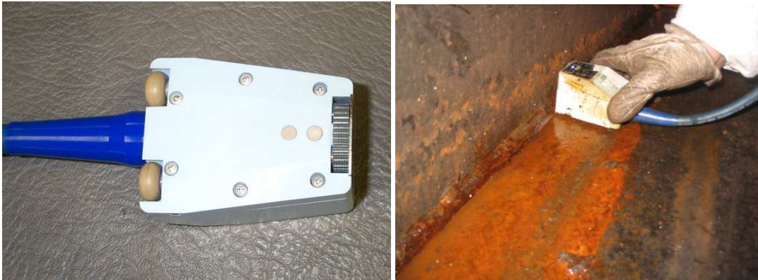
Figure 5. Encoder array probe used to inspect wall to floor weld
