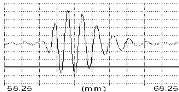
Figure 2: A snapshot of the flaw detector screen showing one HTHA defect
