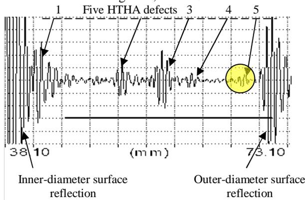
Figure 1: Snapshot of the flaw detector screen showing 5 HTHA defects located along the wall thickness.
