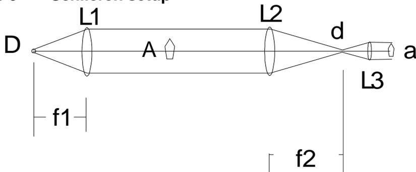
D is the light source. L1 and L2 are the collimating and focusing lenses respectively. “d” is the stop and “a” is the observer located after the magnifying lens L3.
