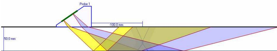
Ray Tracing with pulse mode and divergence effects provide a simple approach to the complexities of mode conversion and complex geometries. Ray Tracing models do not consider diffraction effects therefore the effect is to greatly increase the speed of the calculations and still provide an informative display. Figure 11 from I3D illustrates multiple skips of a divergent beam in a water-filled tube with a 5mm wall.
