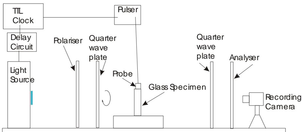
Polarised light is passed through the sample and the light reaching the observer is “nulled” by a second polariser (the analyser). Stresses in the sample then rotate the incident polarised light and are no longer “nulled” when they reach the analyser. These pass through the analyser and are visible to the observer.
