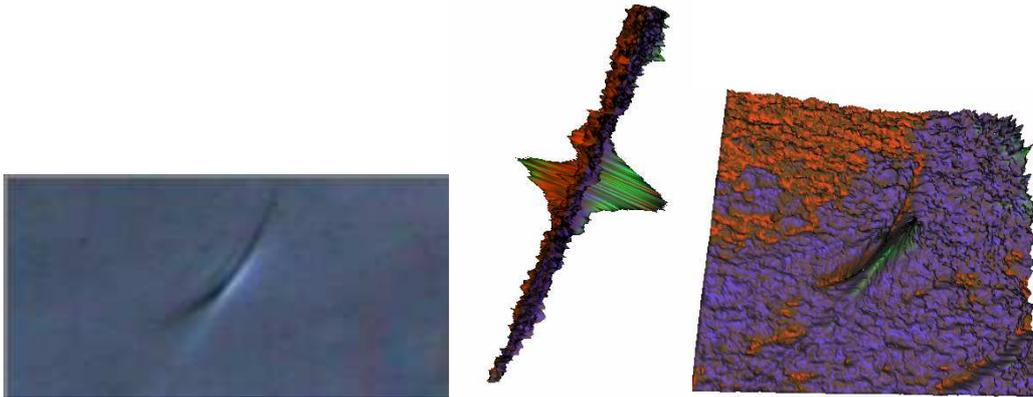
Using the intensities mapped by the image, quantitative assessments of beam size can be made. Computerisation and digital processing make this a much easier and more accurate method than the photodiode displacements proposed by Hanstead. (See Figure 20)
