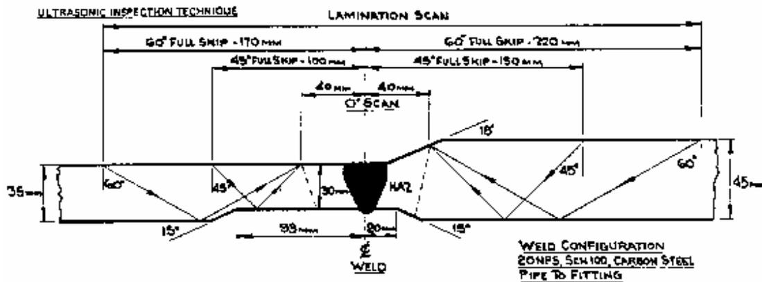
These simple line drawings sufficed for decades. By producing scale drawings and assuming the beam followed simple straight lines it was even possible to predict the locations where mode conversion would occur (such as at the counterbores in Figure 1).
