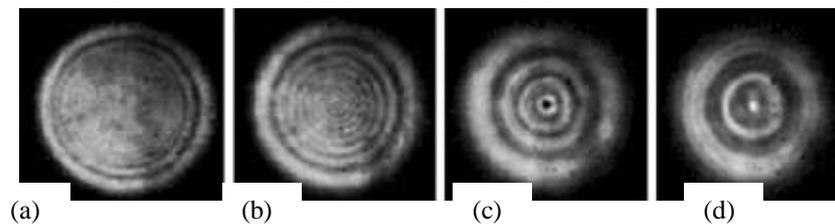
Ultrasonic field of a 5MHz, 25mm diameter, disk-type unfocused transducer at various distances from the radiating surface: (a) 1.65cm; (b) 3.0cm; (c) 6.75cm; and (d) 10.5cm
