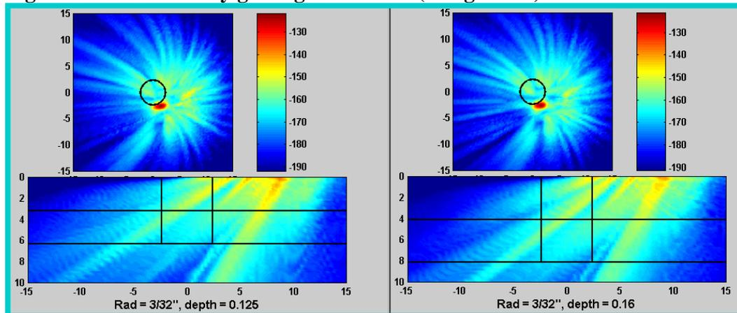
3/16-in.-diameter fasteners on 0.125-in. skin (left) and 0.160-in. (right)
