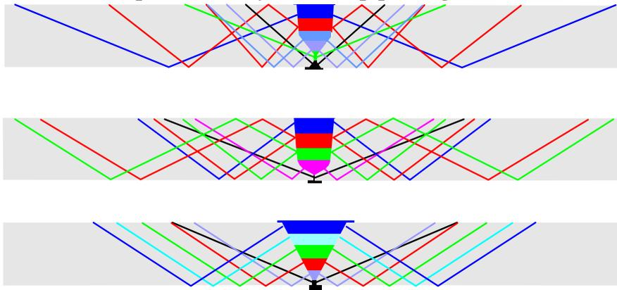
The original multi-probe systems attempted to select focused probes that would be focused at, or as close as possible to, the fusion face. With the introduction of phased array technology the ability to achieve focus at the fusion line was no longer an approximation and zone discrimination was greatly improved.
