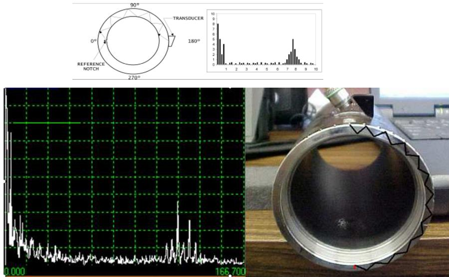
In addition to this issue, the measurement of signal position as a simple relationship between sound-path and circumference is not possible. The pipes in the area of concern were bent to form elbows. This results in a thinning of wall on the extrados and a thickening of the wall on the intrados. This left an elliptical shape with wall thicknesses varying from 5mm to 9mm. A sectioned piece from a removed sample is presented on a scale in Figure 20.
