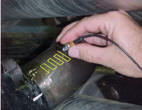
The detection method proposed used a multi-skip transverse wave directed around the circumference of the pipe that was intended to detect the inside and outside surface-breaking flaws. The process worked well on EDM notches and the inspection technique was continued as part of the periodic inspection programme.
