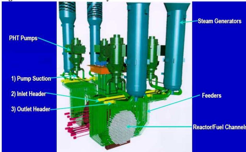
Heavy water is used as both the neutron flux moderator and as the heat transport fluid. The heat transport heavy water is fed into and out of the fuel channels via the Feeders, seen in Figure 17.
