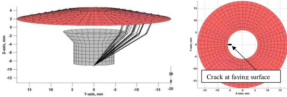
The beam (left image in Figure 3) is designed to be directed tangential to the fastener faying surface so as to strike the potential crack face perpendicularly.
