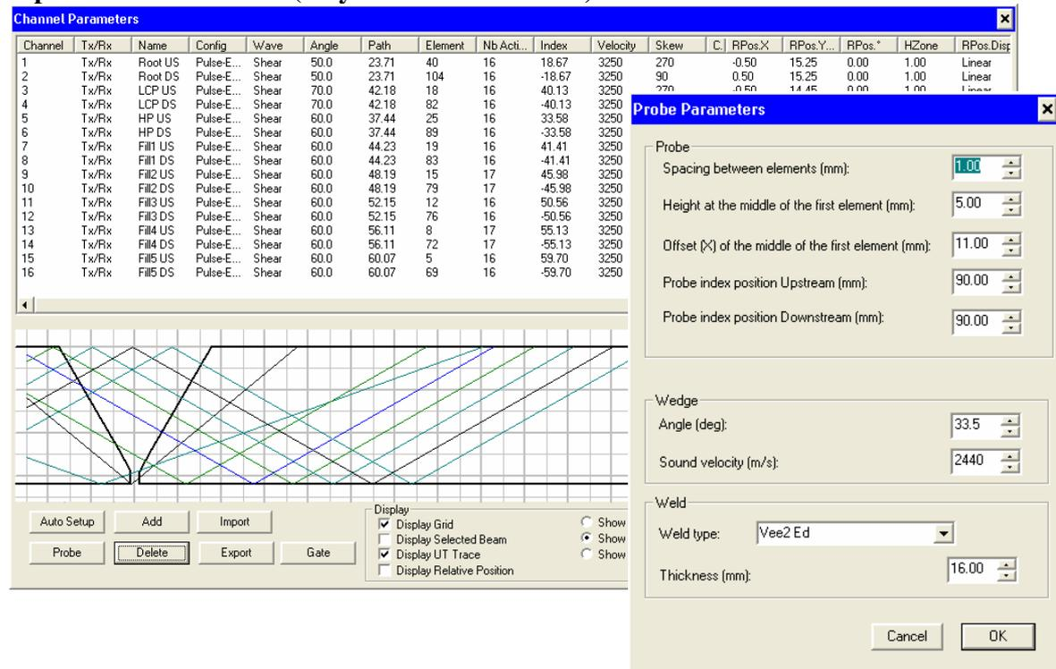
Prior to this phased array modelling feedback tool, the users of multi-probe systems would use Excel spreadsheets to calculate the “ideal” exit point and then use a ruler to position probes. Then they would still need to use a small hammer and tap the probes forward and back to optimise the signal. The manual multi-probe process could take 10-12 hours (and sometimes more) whereas the modelled phased array positioning reduces the calibration setup time to about 2 hours.
