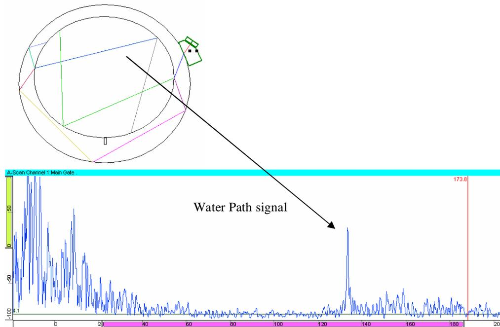
Origin of the multiple arrivals seen at the target notches could be understood once the modelling was used to illustrate the effect of beam divergence. After 2 or 3 skips the divergence provides a “W” shaped pulse moving within the wall. The W shape and the transfer of pulses to the internal water are illustrated in the modelling shown in Figure 23.
