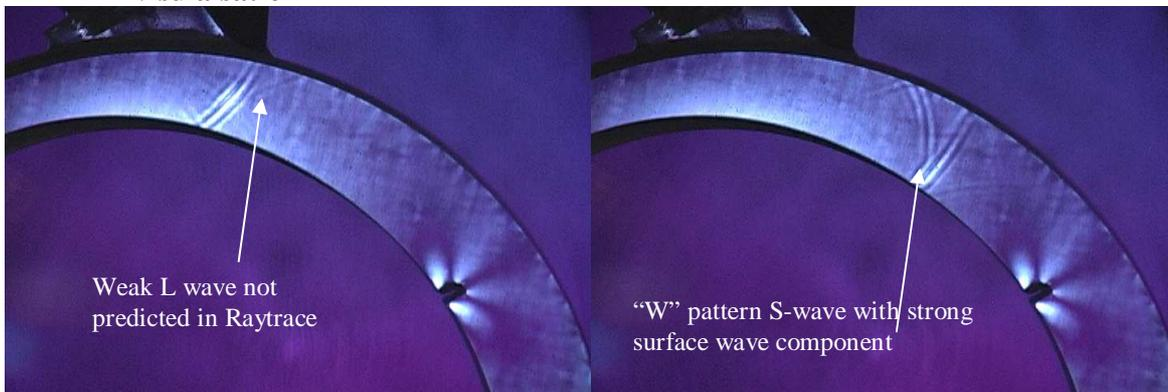
Transmission of the pulse into light water was possible to illustrate with the photoelastic modelling, however, the signals were difficult to see in the water due to a much smaller intensity and shortening of the wavelength. As a result it was not considered useful to further develop the immersion experiment using heavy water. The weak signals from the transmission of pulses from the glass to the light water are seen for two skip points in Figure 24.
