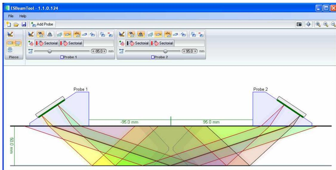
More elaborate modelling options linked to the phased array focal law setups are provided by the manufacturers. ONDT (Olympus NDT) has developed the Advanced Focal Law calculator and Harfang Microelectronics provides their Phase FX software for modelling the beamforming delays and resultant focalisation. They are ideal (and absolutely necessary) when the array is a 2D array with steering in more than one plane.
