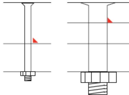
Faying Surface Corner Cracks in Fastener of two sizes: (a) small head/thick skin; (b) large head/thin skin
