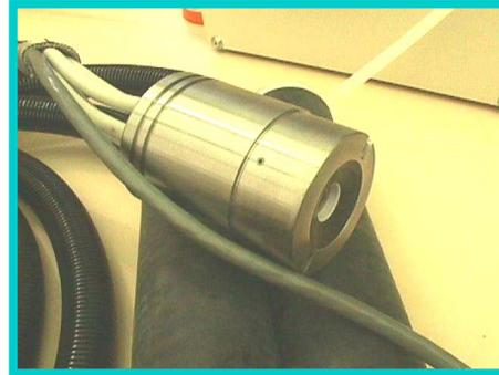
The array output was pre-modelled for its beam characteristics using PASS (Phased Array Simulation Software). The results indicated that the randomness was suitable to reduce the grating lobes.
