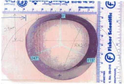
Simple modelling of a pipe with concentric ID and OD and using a single 45° centre of beam ray was therefore not suitable to explain the observed signals.
