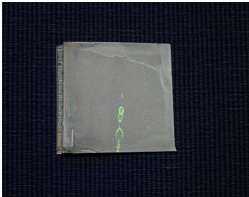
Fig 2(b). Showing grain boundary cracks in Fluorescent DPT.
