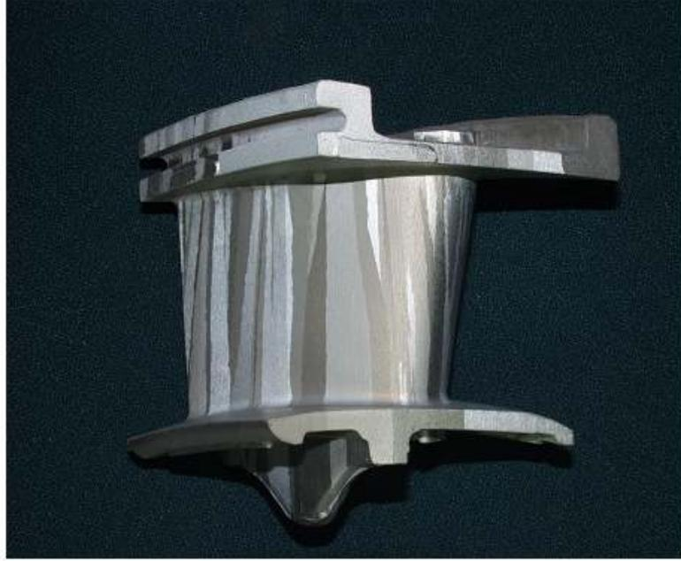
**Fig. 1. High Pressure Turbine Vane showing columnar grains after etching**
