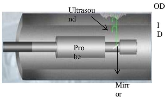
Fig. 4: IRIS Inspection Principle
