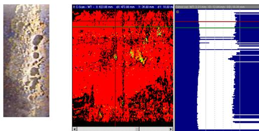
Fig. 6: A One millimeter diameter Pitting Corrosion detected and sized by an RD-Tech IRIS system
