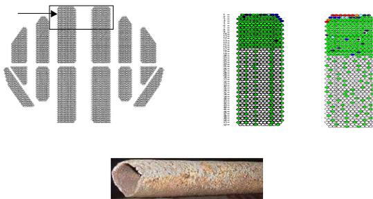
Fig. 8: Corrosion detected and sized by RFEC in a surface condenser
