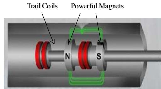
Fig. 3: MFL Inspection Principle
