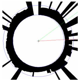
Fig. 7: Under baffle corrosion and external thinning detected by an RD-Tech IRIS system
