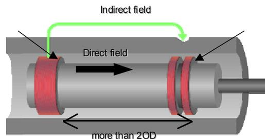
Fig. 2: RFEC Inspection Principle
