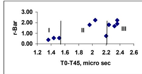
Fig. 7:  $r\text{-Bar}$  plot of the test samples for different values of  $T_0\text{-}T_{45}$  indicating (a) Zone-I Unrecrystallised (b) Zone-II Partially recrystallised and (c) Zone-III Fully recrystallised
