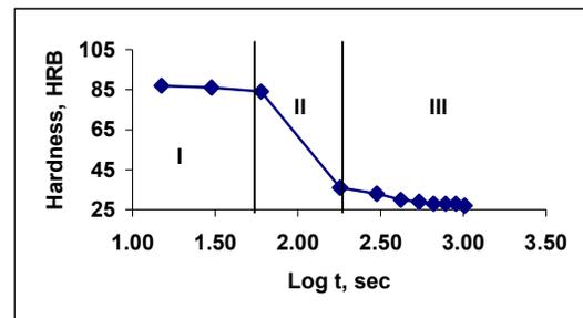
Fig. 1: Hardness plot of the test samples for different logarithmic soaking time scale at  $650^0$  C in a salt bath indicating (a) Zone-I Unrecrystallised (b) Zone-II Partially recrystallised and (c) Zone-III Fully recrystallised
