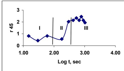
Fig. 4:  $r_{45}$  plot of the test samples for different logarithmic soaking time scale at  $650^{\circ}\text{C}$  in a salt bath indicating (a) Zone-I Unrecrystallised (b) Zone-II Partially recrystallised and (c) Zone-III Fully recrystallised
