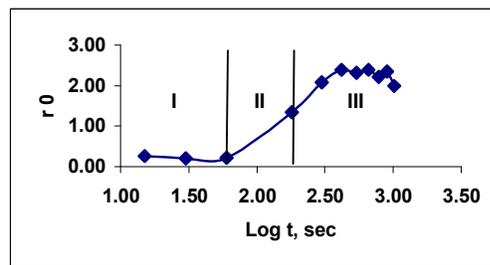
Fig. 3: r0 plot of the test samples for different logarithmic soaking time scale at 650<sup>0</sup> C in a salt bath indicating (a) Zone-I Unrecrystallised (b) Zone-II Partially recrystallised and (c) Zone-III Fully recrystallised
