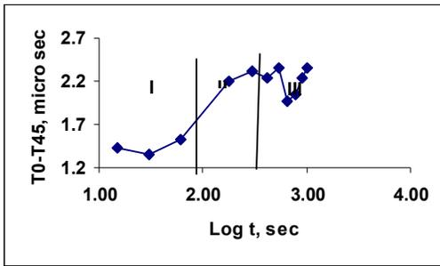
Fig. 2: T0-T45 plot of the test samples for different logarithmic soaking time scale at 650<sup>0</sup> C in a salt bath indicating (a) Zone-I Unrecrystallised (b) Zone-II Partially recrystallised and (c) Zone-III Fully recrystallised
