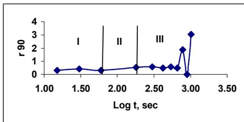
Fig. 5:  $r_{90}$  plot of the test samples for different logarithmic soaking time scale at  $650^{\circ}\text{C}$  in a salt bath indicating (a) Zone-I Unrecrystallised (b) Zone-II Partially recrystallised and (c) Zone-III Fully recrystallised
