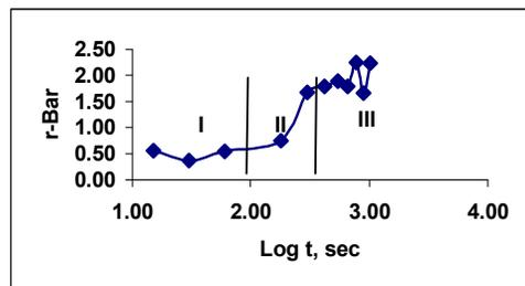
Fig. 6:  $r\text{-Bar}$  plot of the test samples for different logarithmic soaking time scale at  $650^{\circ}\text{C}$  in a salt bath indicating (a) Zone-I Unrecrystallised (b) Zone-II Partially recrystallised and (c) Zone-III fully recrystallised
