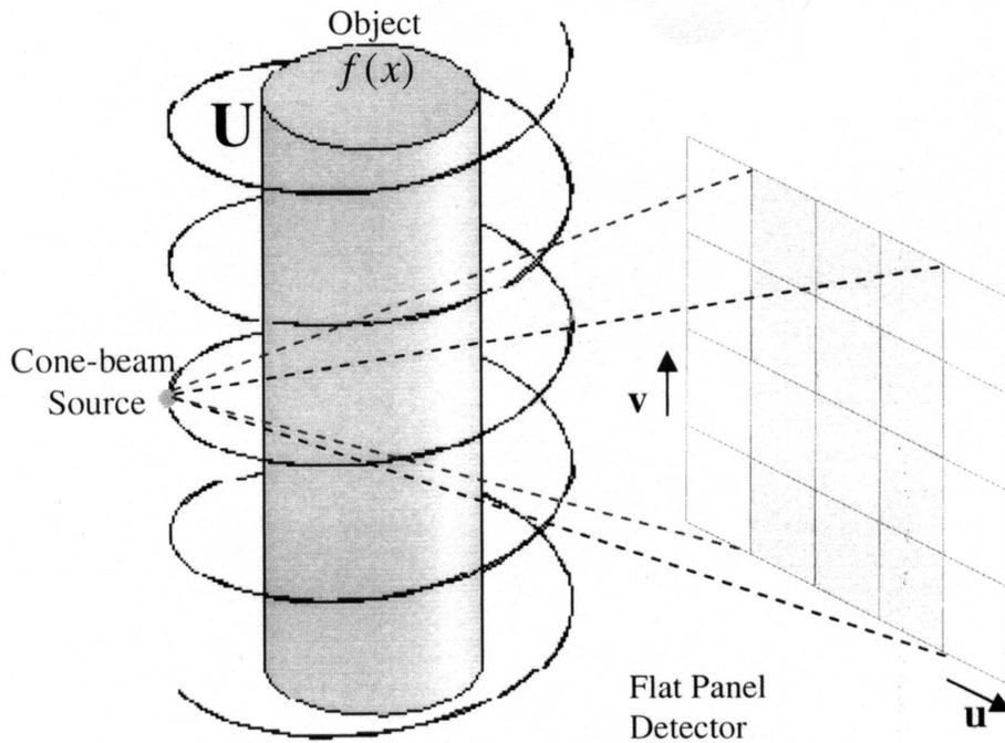
Fig. 1: Projection Truncation in 3D helical scanning
