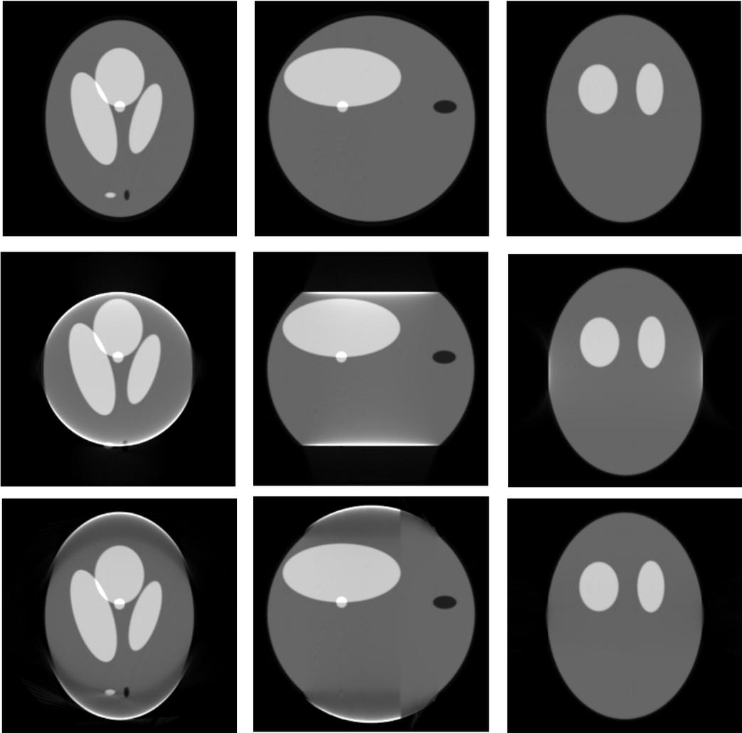
Fig. 4: Reconstruction of high contrast Shepp-Logan Phantom, 55 detectors are truncated in the detector plane on either side. The first row - complete projection data, the second row - truncated projection data and the third row - projection completion using linear prediction. Left column shows the slice at  $z = -0.25$ , the middle shows slice at  $y = 0$  and right column shows slice at  $x = 0$ . The gray scale window used is  $[0.0 \ 2.5]$
