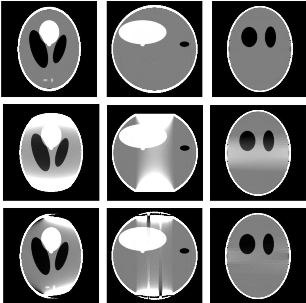
Fig. 3: Reconstruction of low contrast Shepp-Logan Phantom, 35 detectors are truncated in the detector plane on either side. The first row - complete projection data, the second row - truncated projection data and the third row - projection completion using linear prediction. Left column shows the slice at  $z = -0.25$ , the middle shows slice at  $y = 0$  and right column shows slice at  $x = 0$ . The gray scale window used is  $[1.0 \ 1.04]$ .
