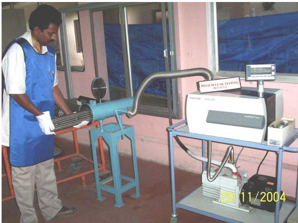
Helium leak Testing of Fuel Bundle
