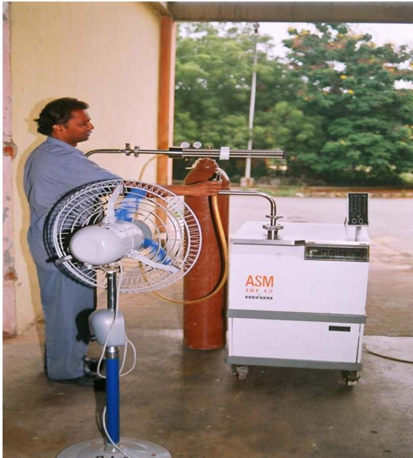
Helium leak testing of appendage welded Fuel tubes
