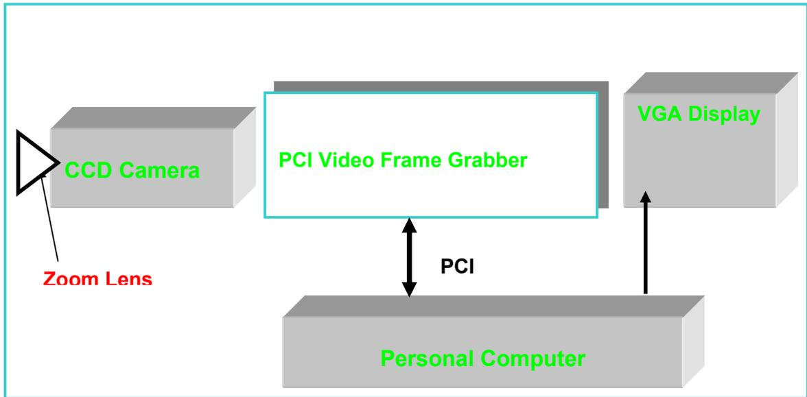
Fig. 6 Schematic Diagram of Vision System showing various components.
