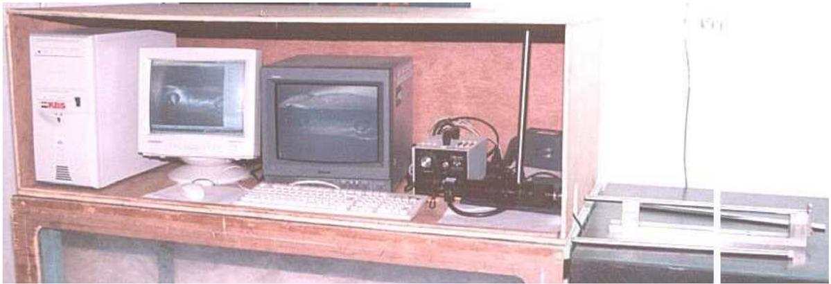
**Fig.8 Vision system for Tube inspection**
