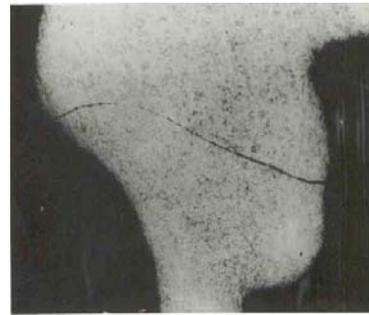
Fig.7b Weld with lack of fusion
