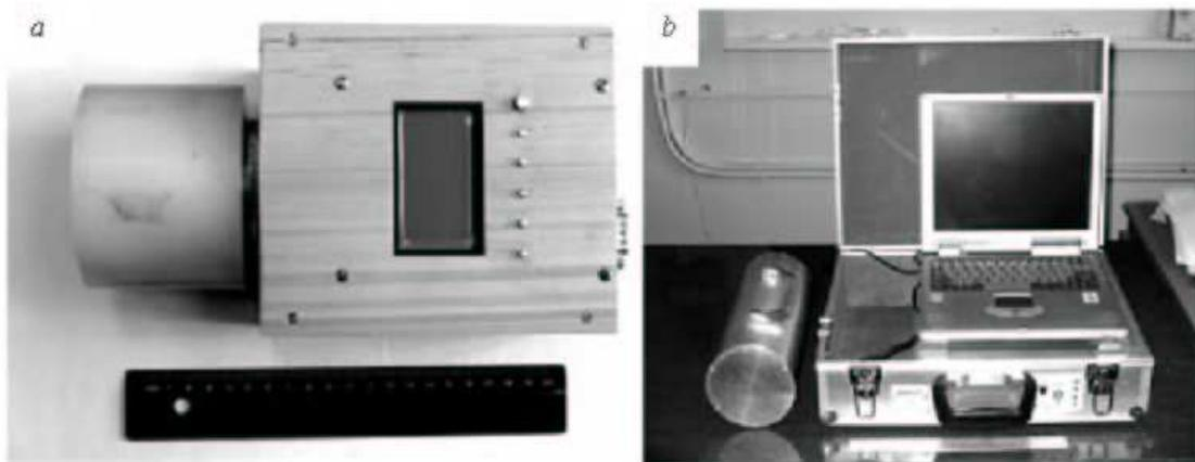
Fig. 5: (a) Neutron detector on the base of  ${}^6\text{Li}$ -glass scintillator and (b) Gamma-spectrometer “PEGAS”
