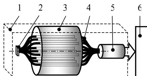
Fig. 2: Scintillation detector of neutrons
