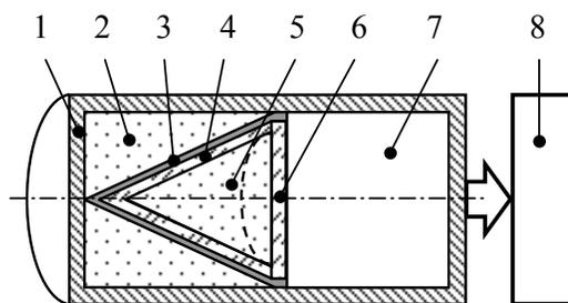
Fig. 1: Scintillation detector of neutrons
