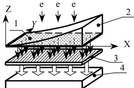
Fig. 3: Scintillation sensor for electron and  $\beta$ -radiation
