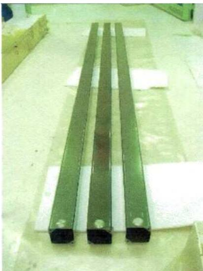
Fig. 2: TAPS square channels developed by NFC in seamless route
