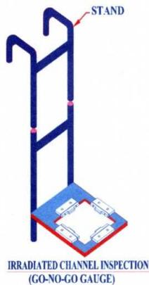
Fig. 5: General arrangement of go- no-go gauge
