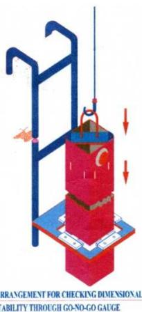
Fig. 6: Irradiated fuel channel testing in the gauge
