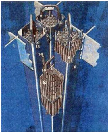
Fig. 1: General arrangement of fuel I assembly channel & control blade
