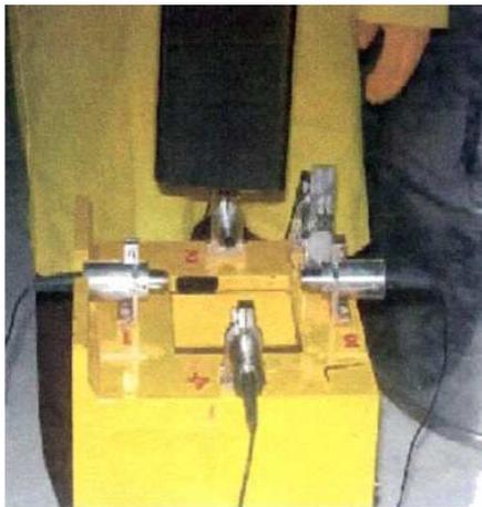
Fig. 7: UT probes (4) mounted on probe holder
