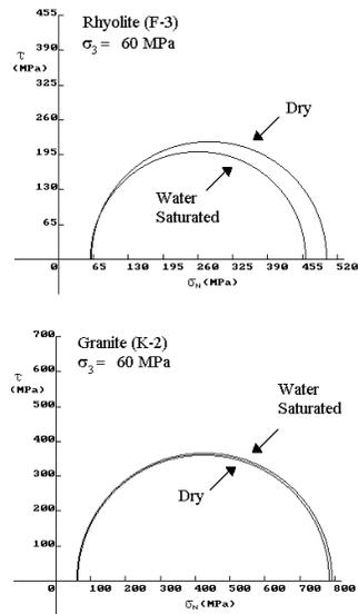
Fig. 2: Mohr's circles drawn from the triaxial compression stress data of dry and water-saturated rhyolite (F-3) and granite (K-2)
