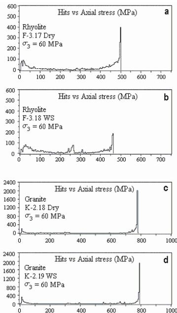
Fig. 3: Hard copies of the graphs showing the occurrence rate of AE hits plotted against the axial stress in dry and water-saturated samples of rhyolite and granite. The tests were carried out at 60 MPa confining pressure. The experimental conditions and detection level of AE were kept identical during all these tests.
