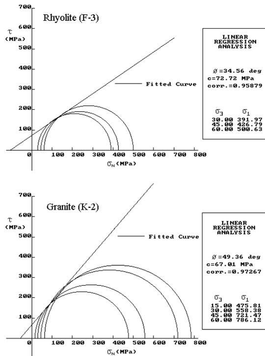
Fig. 1: Mohr's circles, Mohr-Coulomb envelope and the results of 'C' and 'φ' of dry rhyolite (F-3) and granite (K-2).
