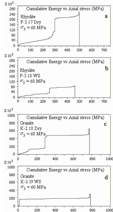
Fig. 4: Hard copies of the graphs showing the cumulative energy of AE counts plotted against the axial stress in dry and water-saturated samples of rhyolite and granite. The tests were carried out at 60 MPa confining pressure. The experimental conditions and detection level of AE were kept identical during all these tests
