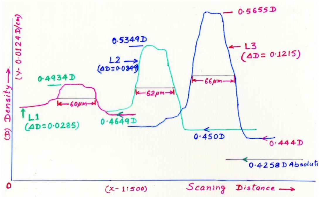
Figure 3: Microdensitometer scan across the image of air gap having variable width
