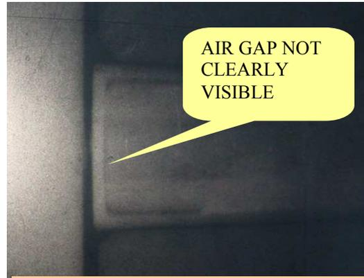
Figure 5: Poor contrast radiograph with masking
