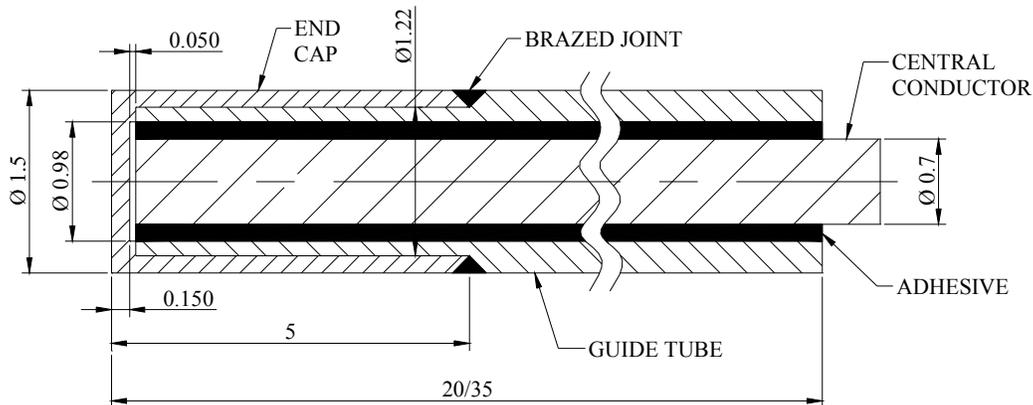
Figure 7 : Sensor (Modified Design)
