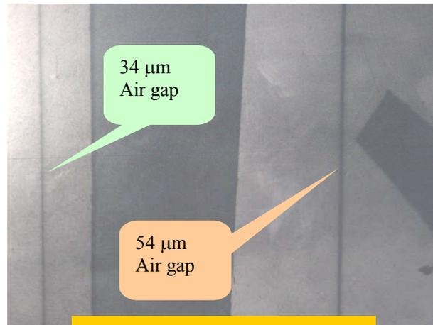
Figure 6: Thick and thin air gap
