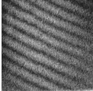
Fig. 8: Interferogram of region with tight crack
