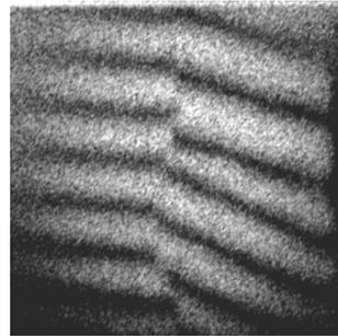
Fig. 6: Interferogram showing fringe discontinuity along crack
