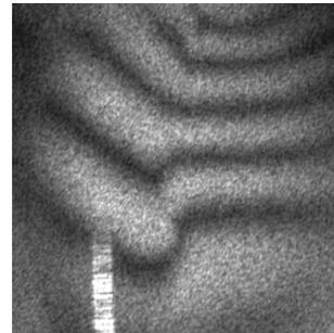
Fig. 7: Interferogram showing fringe discontinuity along crack
