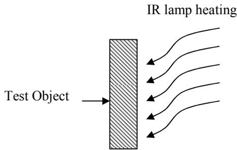
Fig. 4: Thermal loading setup with IR lamp
