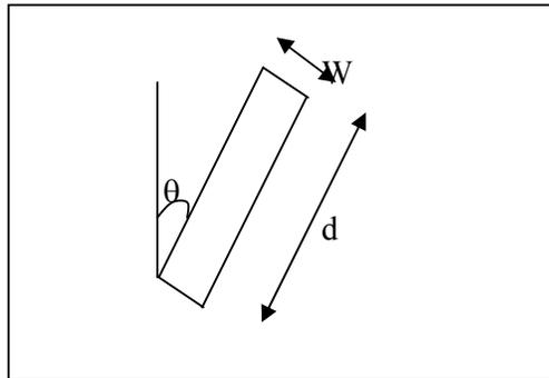
Fig. 1: Crack / Missed joint parameter sketch
