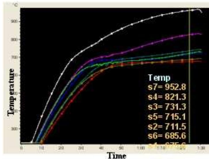
Fig. 3: Temperature profiles of the base plate and TBCs coated plates
