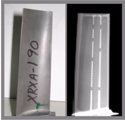
Fig. 1: Photo and Digital Radiograph (DR) of Turbine blade
