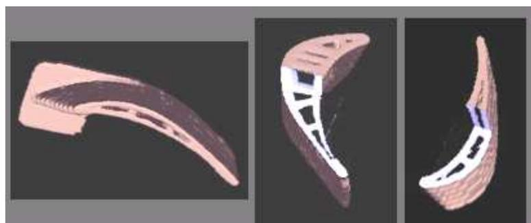
Fig. 4: 3D visualization and its cut-out views of Turbine blade
