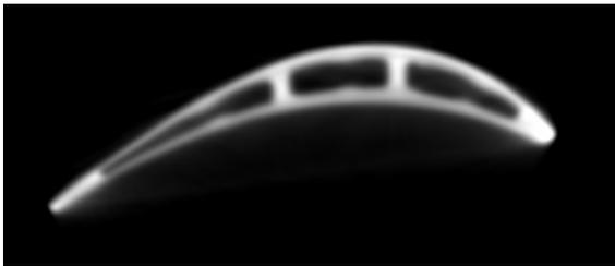
Fig. 2: Tomogram showing the cross-sectional image of the turbine blade
