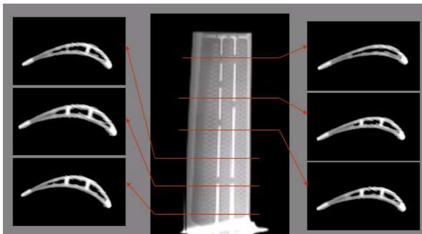
Fig. 3: Tomograms of Turbine blade at different locations selected from DR
