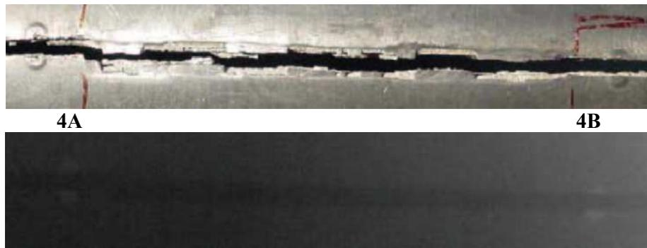
Fig. 11: Photograph of the crack through blisters 4A and 4B in the burst pressure tube (top) and its neutron radiograph (bottom)
