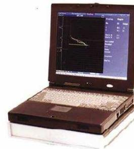
Fig. 1: Technofour's modern portable eddy current tester SD-PC-12
