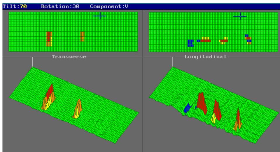
Fig. 14: Color-coded C-Scans showing transverse and longitudinal defects
