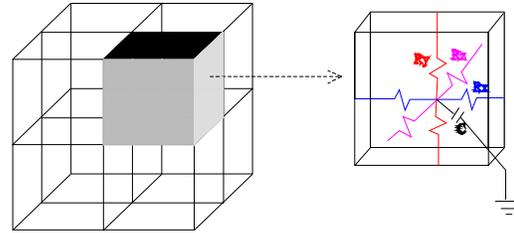
Fig. 3: Three-dimensional equivalent electrical model for heat conduction
