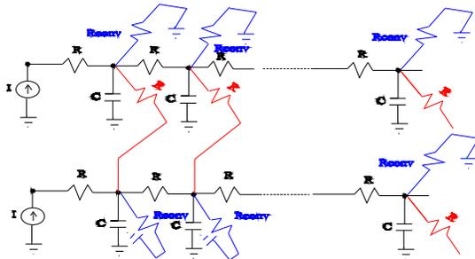
Fig. 2: Two-dimensional equivalent electrical model for heat conduction
