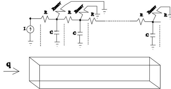
Fig. 1: One-dimensional equivalent electrical model of heat conduction
