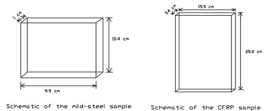
Fig. 4: Dimensional layouts of the (a) Mild steel, and (b) CFRP samples
