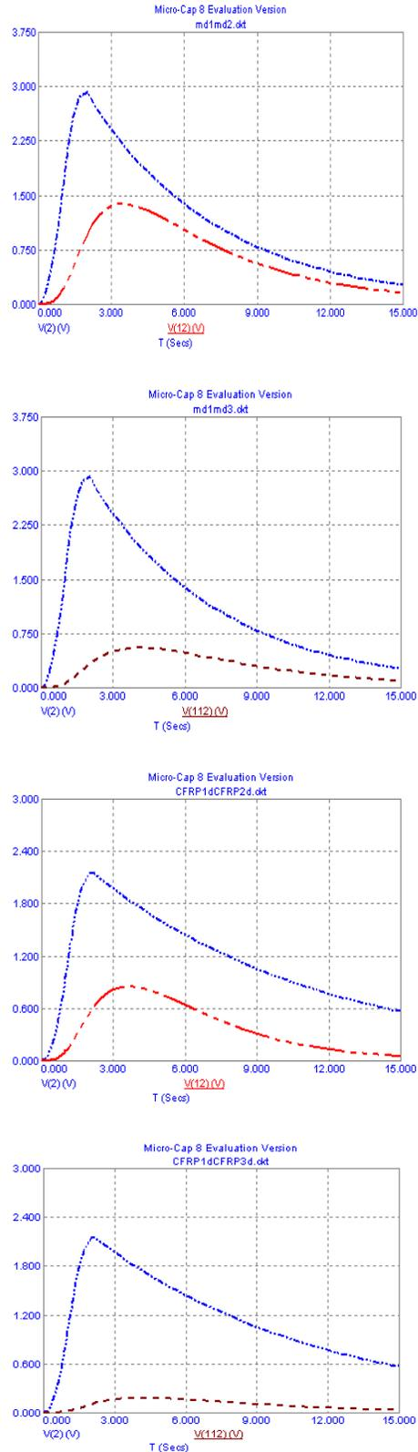
Fig. 5: 1D, 2D and 3D simulation results of mild steel (top two plots) and CFRP
