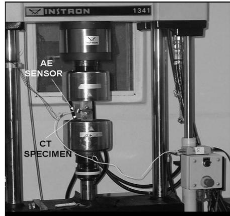
Fig. 2: Laboratory fatigue test set up
