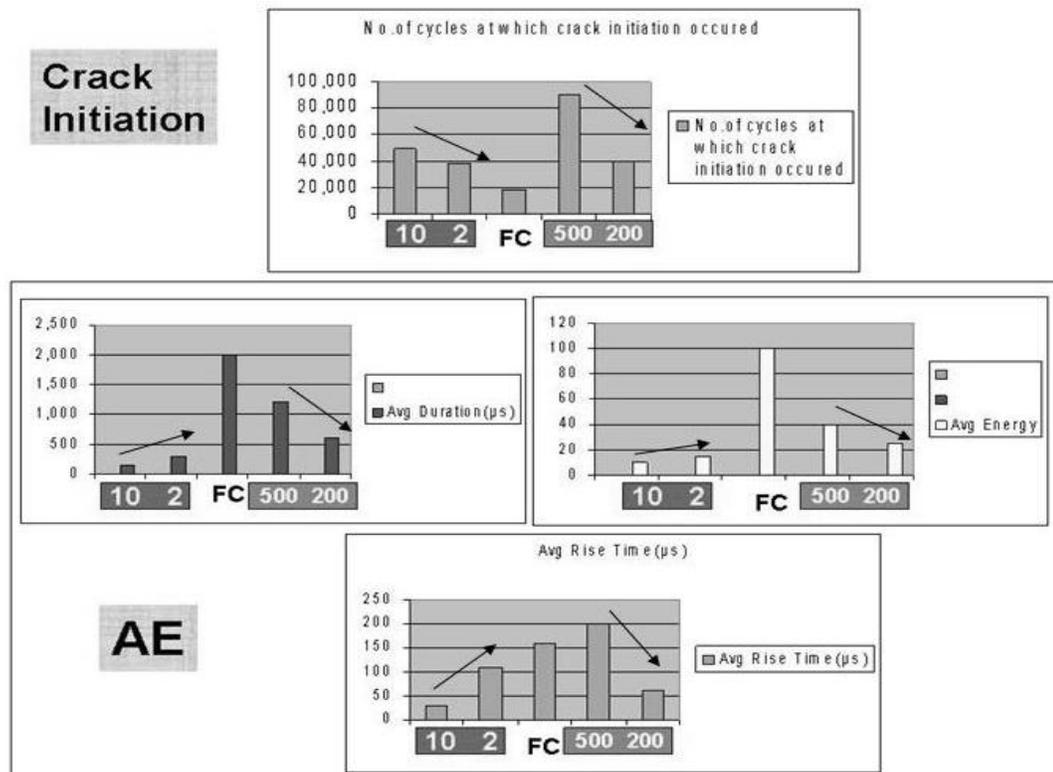
Fig. 6: AE parameters manifest themselves qualitatively so as to discriminate different heat treatment procedures
