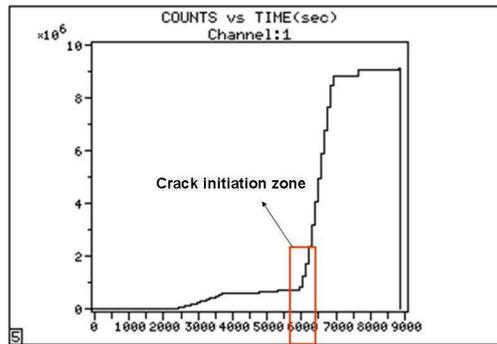
Fig. 3: Plot isolating crack initiation in 12.5 mm sample
