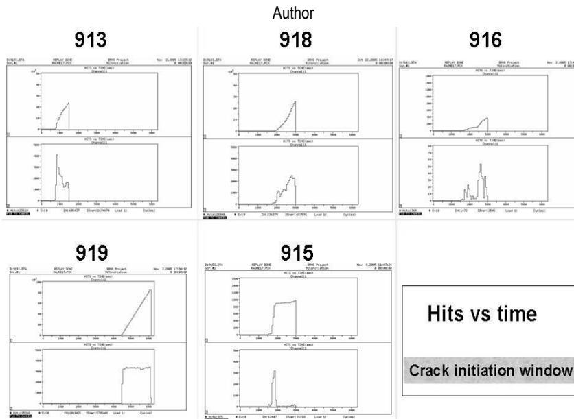
Fig. 4: Acoustic emission hits profile at crack initiation
