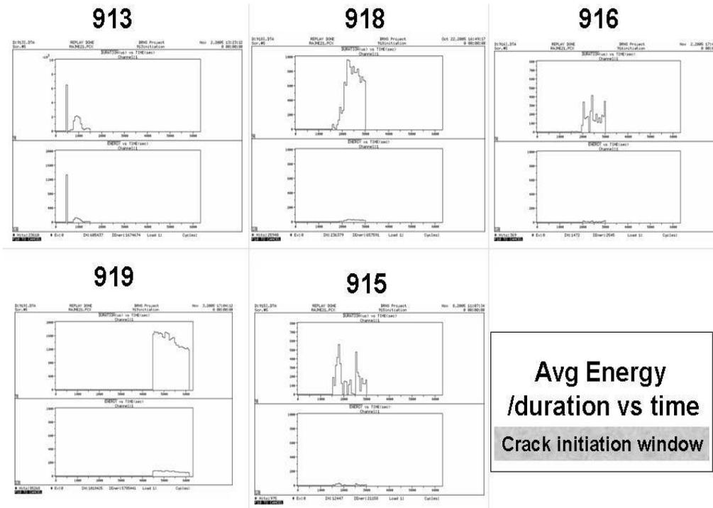
Fig. 5: Acoustic emission energy/duration profile at crack initiation
