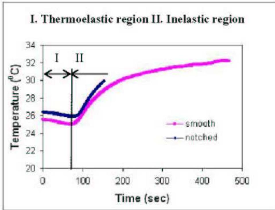
Fig. 5: Temperature-time curve for IMI-834 Ti alloy
