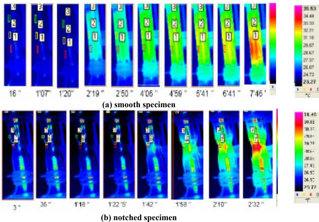
Fig. 4: Thermograms at different time intervals for the IMI-834 Ti alloy
