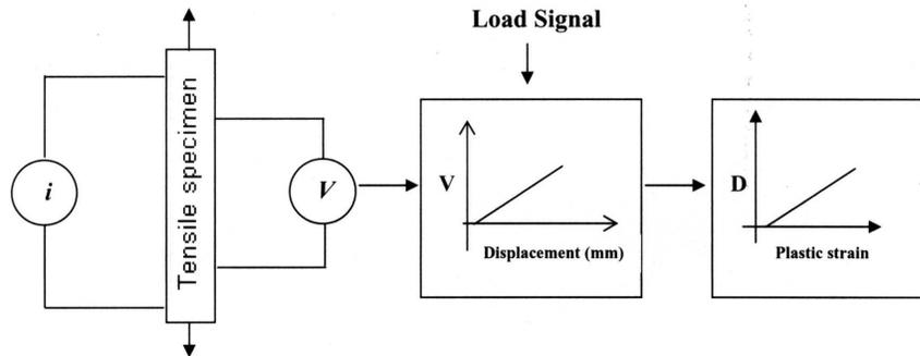
Fig. 1: Schematic diagram of ACPD Technique for damage measurement
