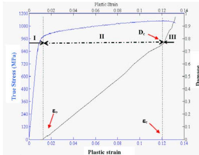
Fig. 2: Damage-plastic strain-true stress curve
