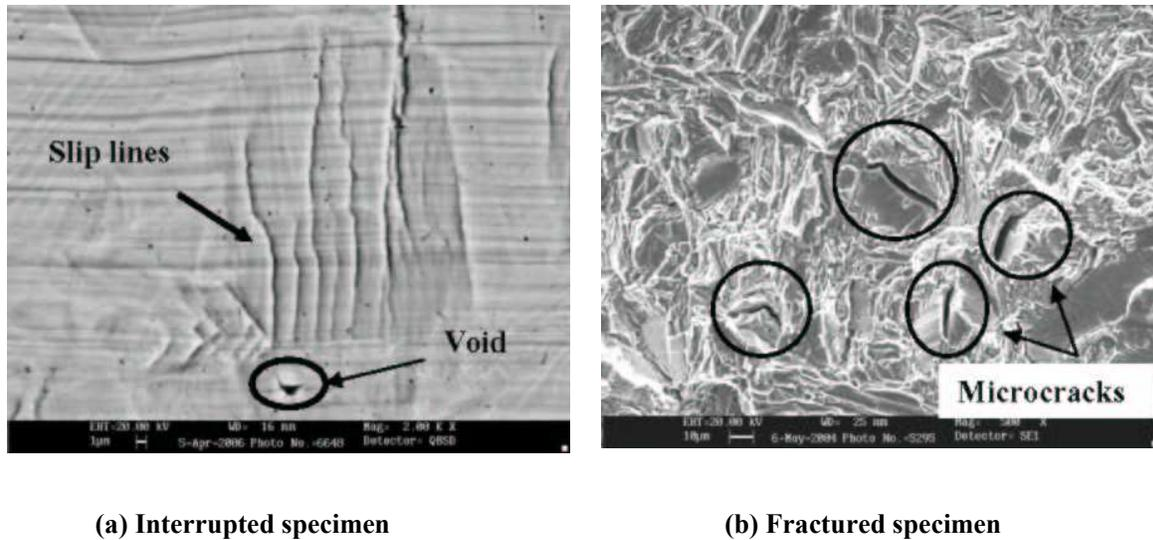
Fig. 7: Damage micromechanism in IMI-834 Ti alloy
