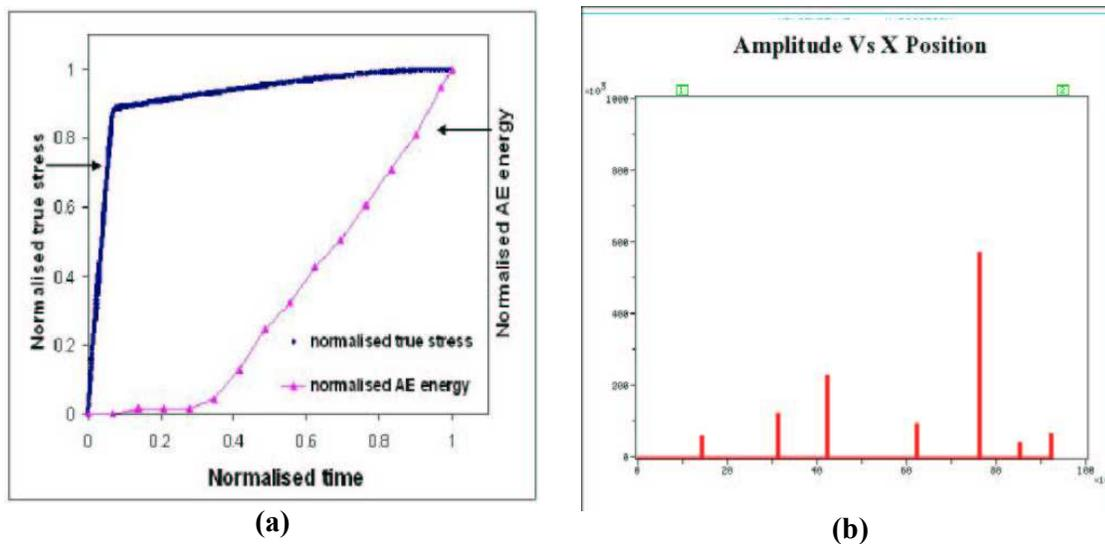
Fig. 3: Typical AE signals for near- $\alpha$  IMI-834 Ti alloy under monotonic loading conditions
