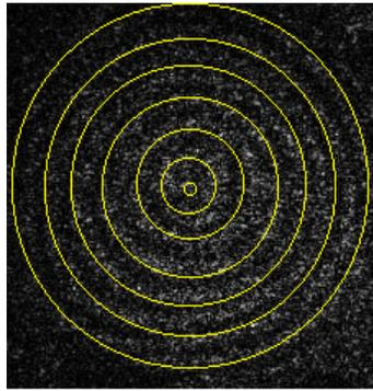
Fig. 4: Fringe pattern generated for a defect free specimen
