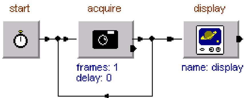
Fig. 2: Data flow diagram for continuous acquisition of images
