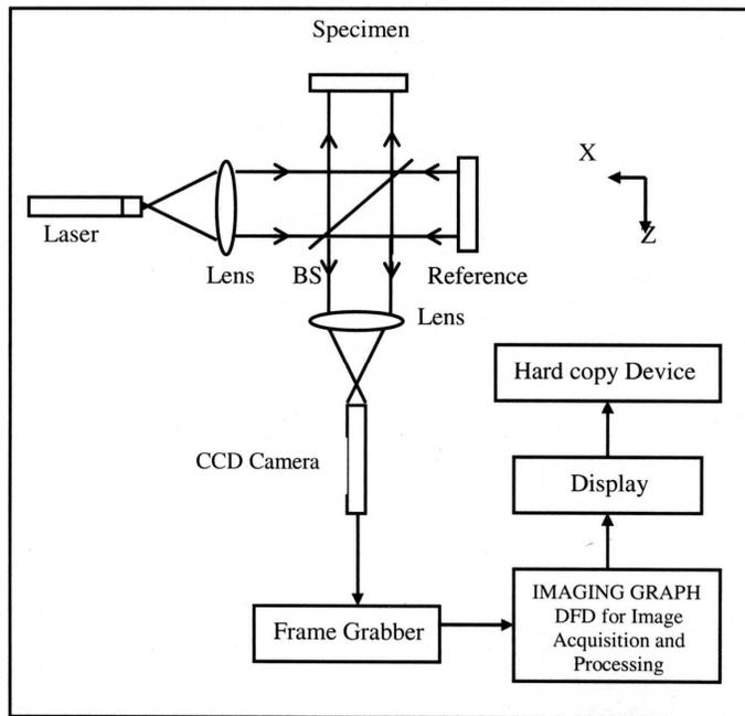
Fig. 1: Lay out of the ESPI system with out of plane optical configuration
