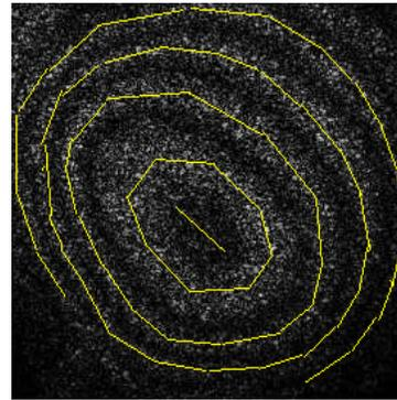
Fig. 5: Fringe pattern generated for a defective specimen
