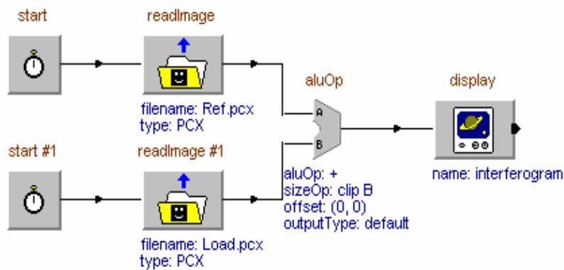
Fig. 3: Data flow diagram for continuous subtraction or addition of images
