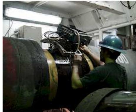
Fig. 5: Pipeline weld scanner
