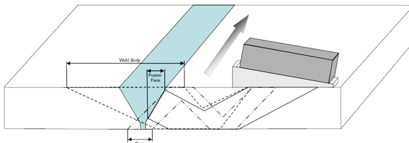
Fig. 6: Single pass weld coverage with phased array
