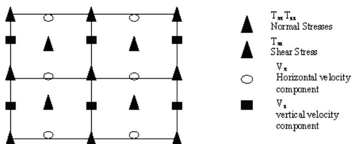
Fig. 2: Finite difference grid of the domain showing the positions of each field variable
