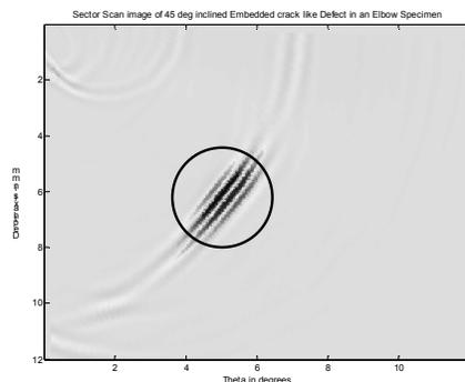
Fig. 7: Sector Scan image of 45 deg inclined embedded crack like Defect in an Elbow Specimen
