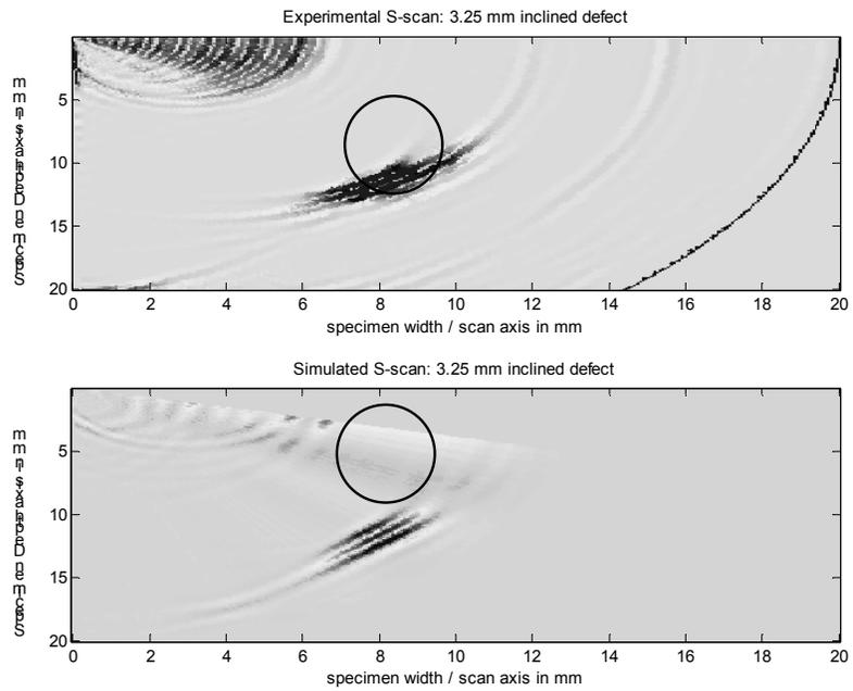
**(a) 3.25 mm Inclined defect**
