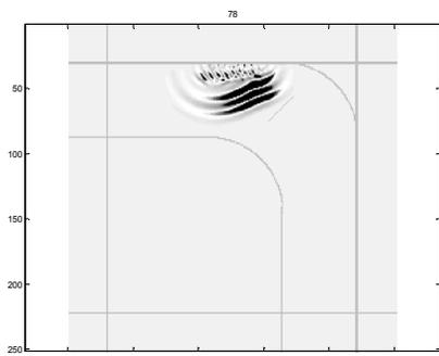
Fig. 6: Phased array wave propagation in an elbow and its interaction with an inclined defect
