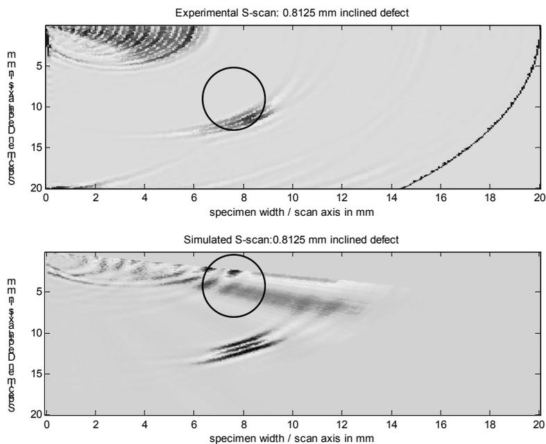
(c) 0.8125 mm Inclined defect
