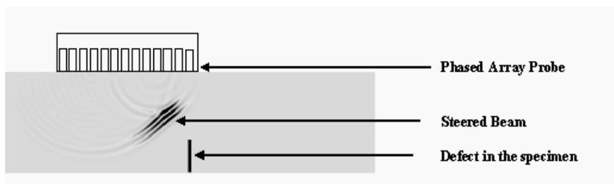
Fig. 1: Beam steering and focusing in a phased array transducer
