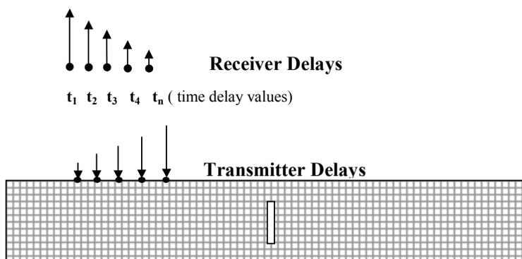
Fig. 3: Finite difference model for phased array transmission and reception
