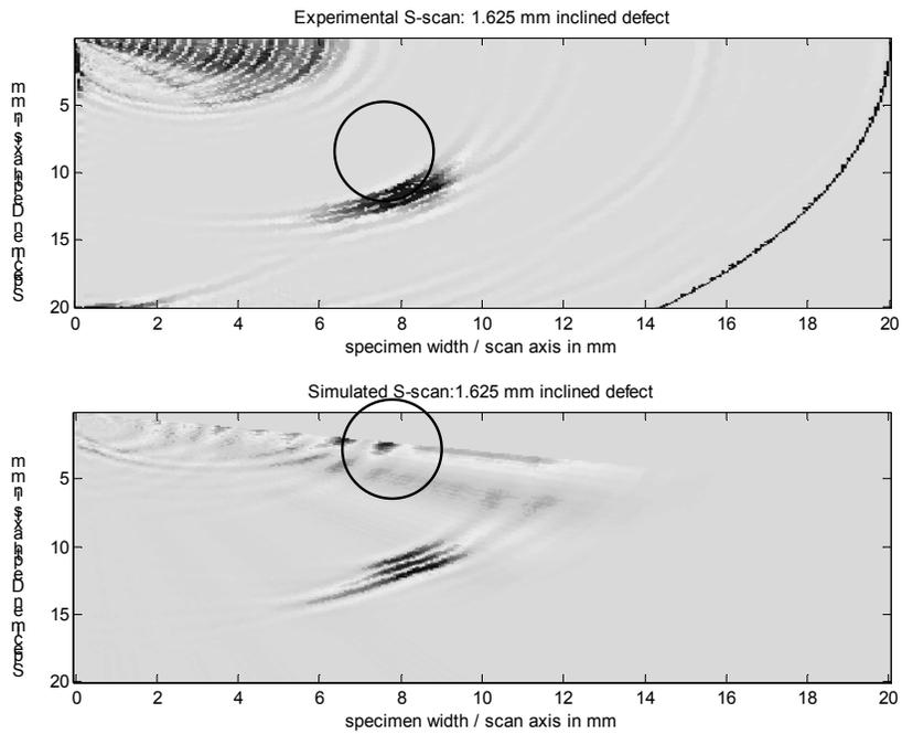
**(b) 1.625 mm Inclined defect**
