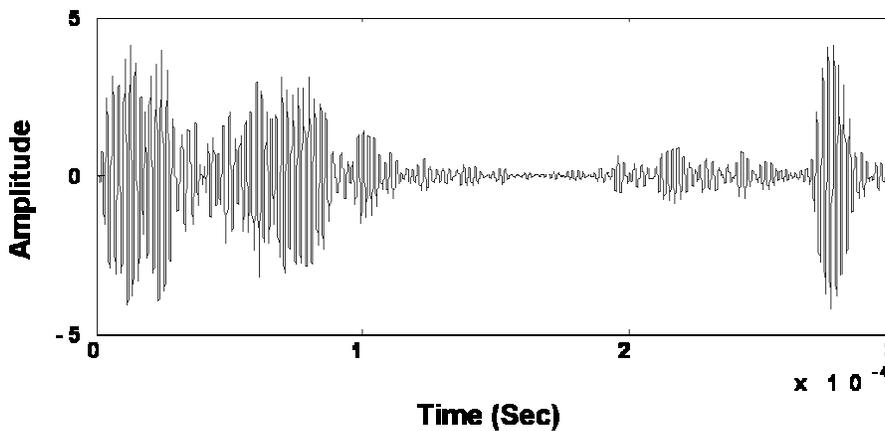
3: A- scan signal of the reflection from Vinyl ester resin interface
