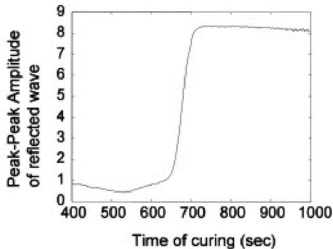
Fig 6: Peak-Peak amplitude of the reflected wave from the vinyl ester resin interface as the resin cures
