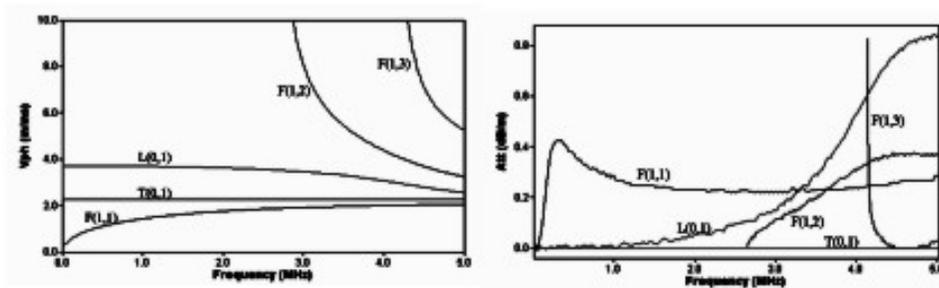
Fig 1: Dispersion curves for wave modes in copper wire of radius 0.25 mm in air plotted using DISPERSE
