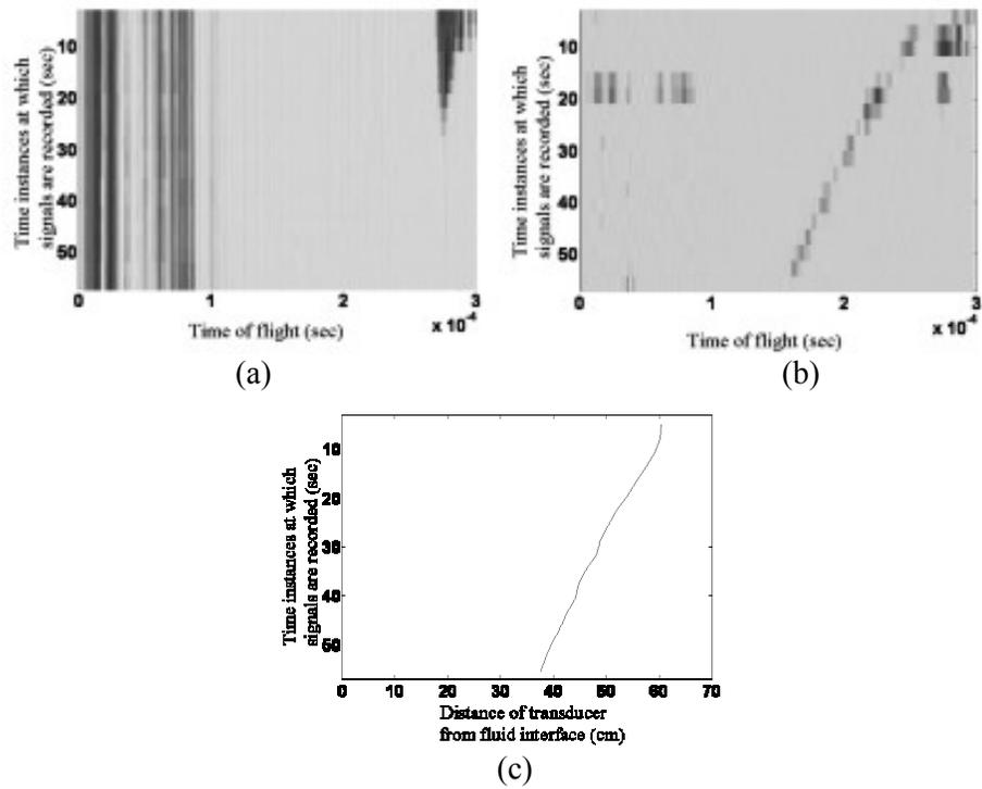
Fig 4: Images for vinyl ester resin. (a) Raw unprocessed B-scan image (b) Processed B-scan image (c) Flow front profile
