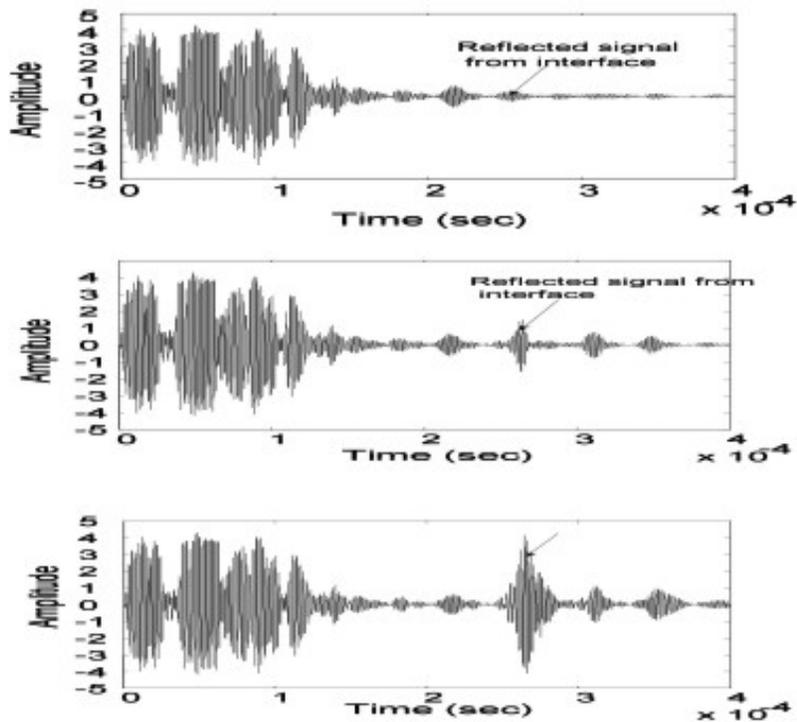
Fig 5: A-scan signals while vinyl ester resin is curing at different time instances of time (a) 9 minutes, (b) 11 minutes, (c) 15 minutes
