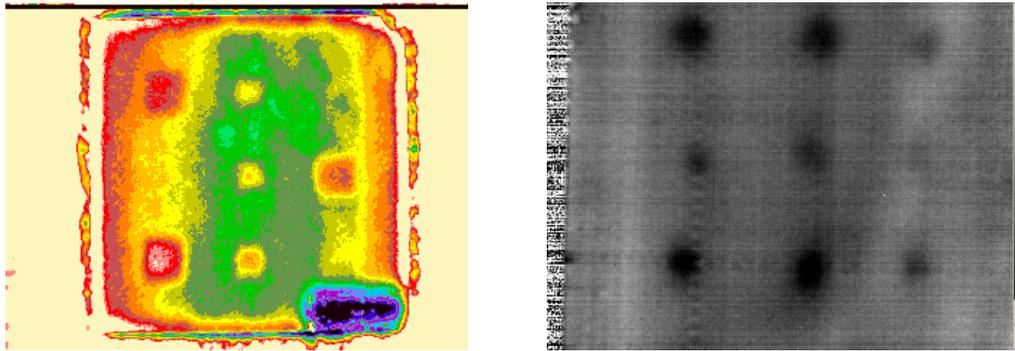
Figure 3 . Honeycomb panel with debonds between face sheet & core by PT
