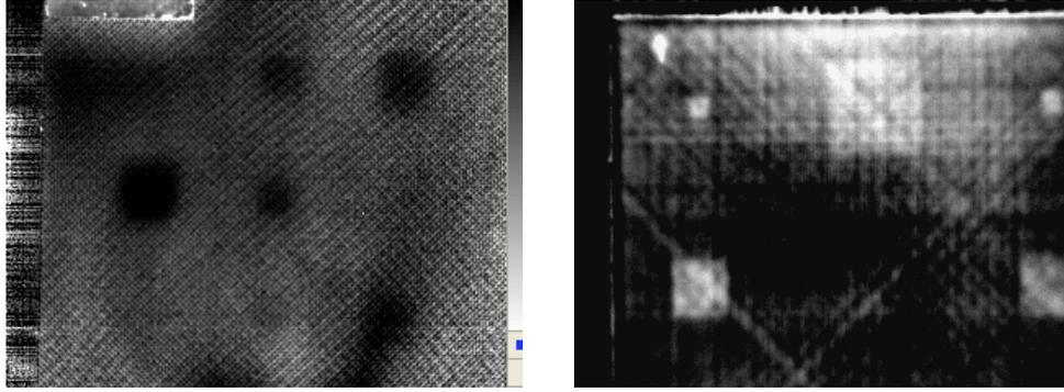
Figure 4 Debonds between the layers in the composite skins of a honeycomb panels by LT
