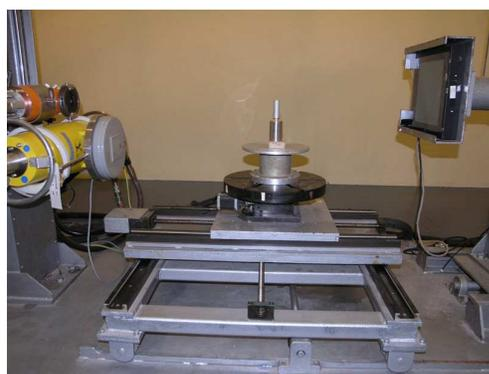
Fig.1: Real-Time DR System consists of X-ray machine, FPD and 4-axis object manipulator
