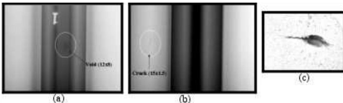
Fig.4: Digital radiographs at two orientations showing (a) void (b) crack and (c) photograph of the Cut cut section showing the real nature of the defect
