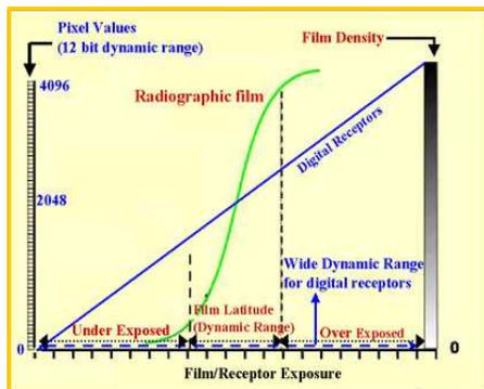
Fig 2: Comparison of response curve for film and FPD
