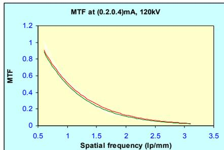
Fig 3: MTF curve of the FPD showing spatial resolution of 2.5 lp/mm
