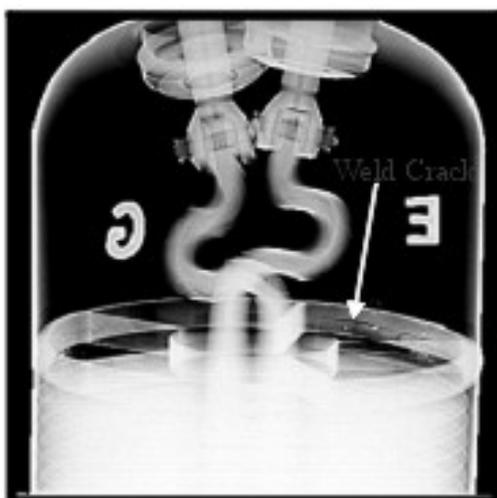
Fig.5: Digital radiograph showing weld crack in a space vehicle component
