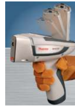
2009:Thermo NITON XL3 1st handheld XRF with 50kV Au anode x-ray tube and automatic parameter optimization
