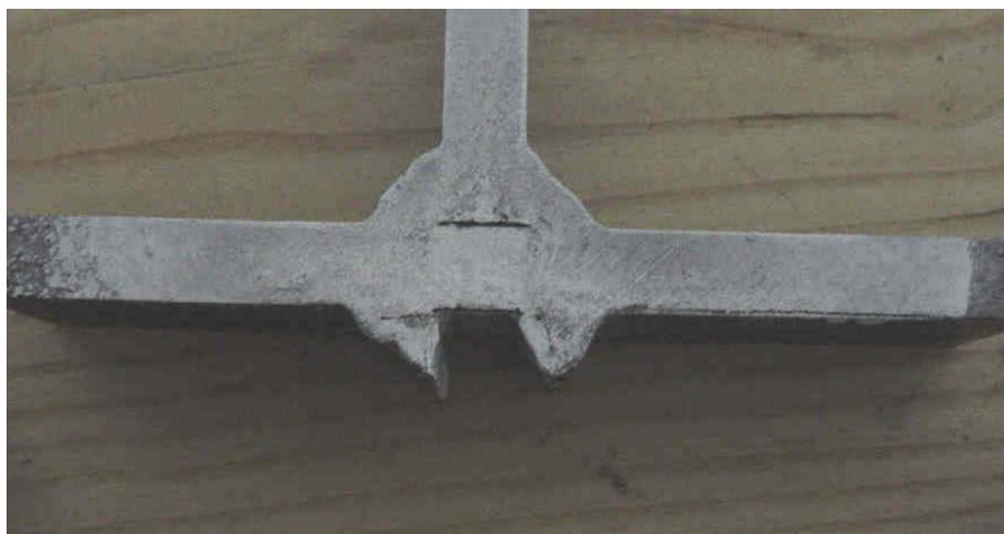
Fig. 1: Frame with cruciform joints failed because of having been only fillet-welded.
