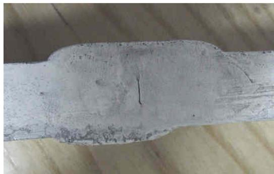
Fig. 4: Macrograph, detection of incomplete penetration.
