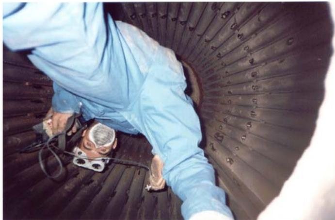
Fig. 4: Ultrasonics thickness measurement of tubes.
