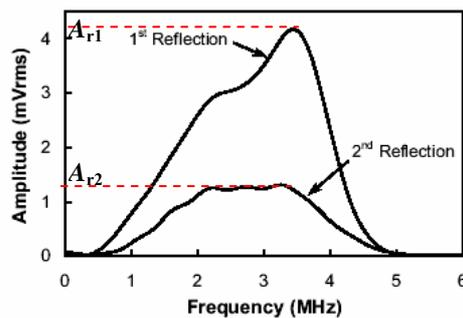
Fig. 7: First and second reflection of measured signal.
