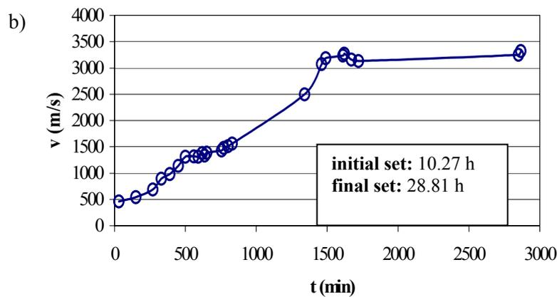
Fig. 3: Velocity in time for a) concrete without admixture (mixture I) and b) concrete with addition of retarder (mixture II).
