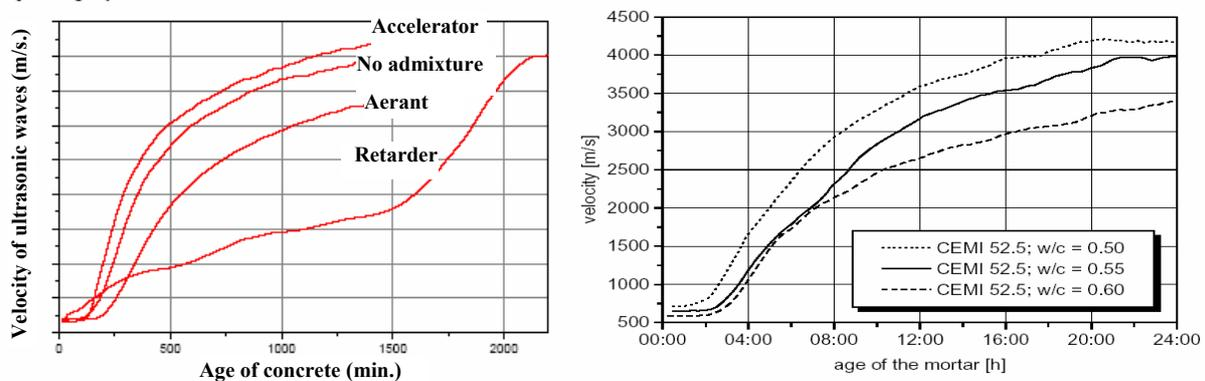
Fig. 4: velocity of P waves dependent on setting and hardening process for a) different admixtures [2] and b) different w/c ratios [3].
