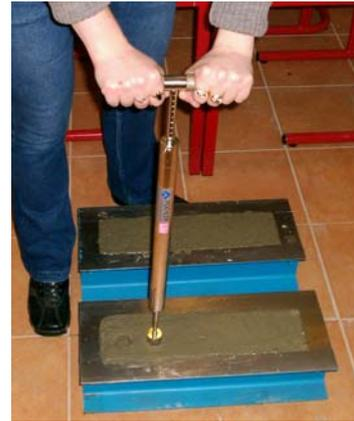
Fig. 2: Ultrasound measurements and setting time determination by means of penetrometer.
