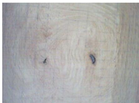
Fig. 7: The image of the plywood with defects.
