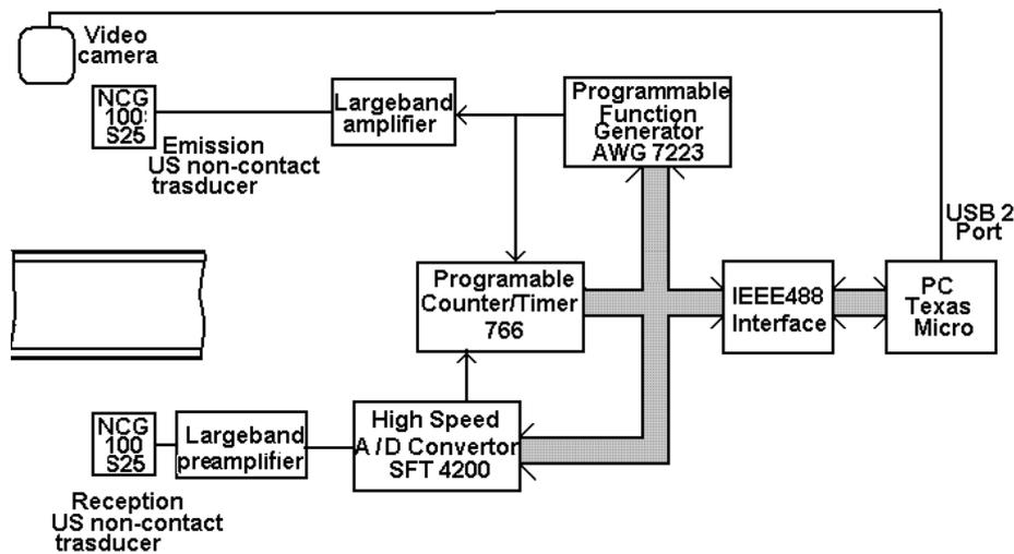
Fig. 4: Experimental set-up.
