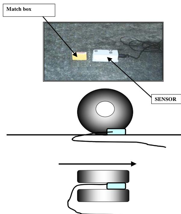
Fig 3: Set up of the FDP sensor.
