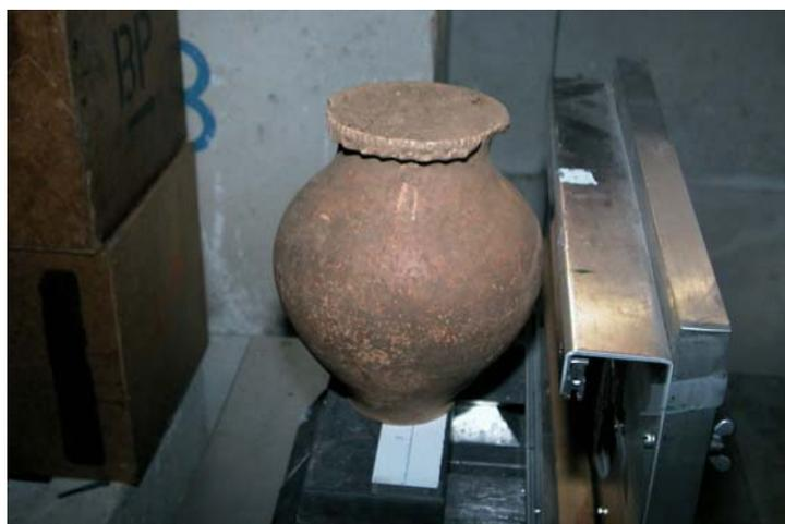
Fig. 1: The photography of the treasure find in a ceramic pot positioned for NR examination in the NR channel of the Ljubljana TRIGA Mark II research reactor.
