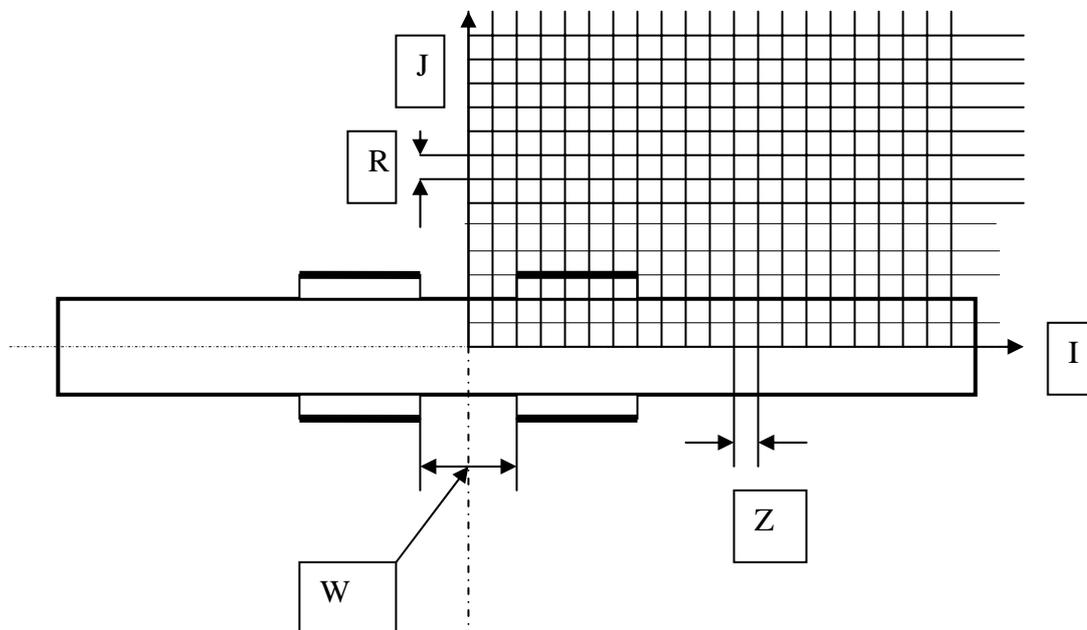
Fig. 2: The mesh points where the vector potential will be calculated.
