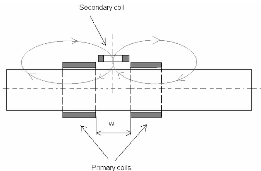
Fig. 1: Primary and secondary coils.
