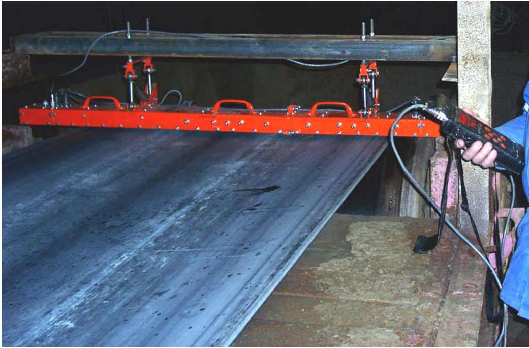
Fig. 1: INTROCON flaw detector on a conveyor.
